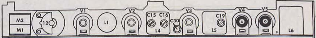
Figure 20. Parts location, Radio Receiver and Transmitter BC-611-B.
