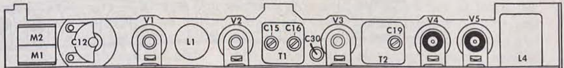
Figure 21. Parts location, early Radio Receiver and Transmitter BC-611-C.
