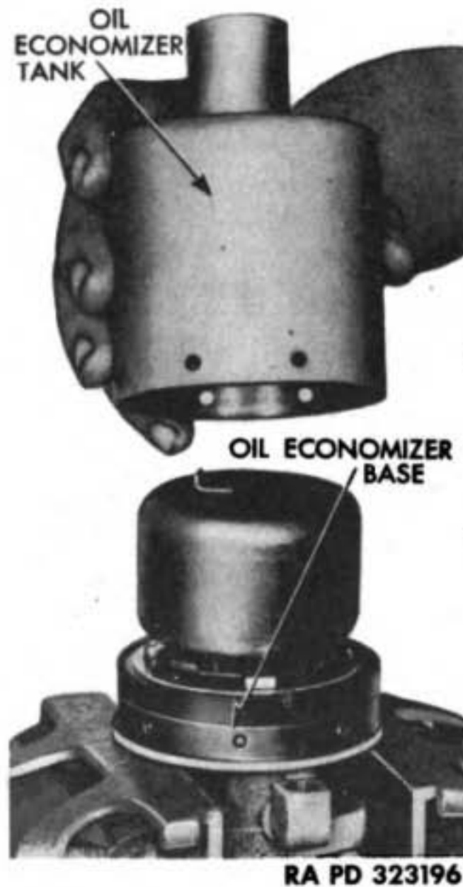
Figure 200 — Removing Oil Economizer Tank
