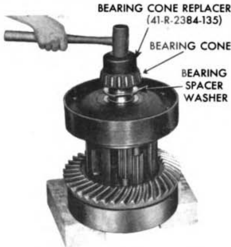
Figure 102 — Installing Differential Bearing Cone
