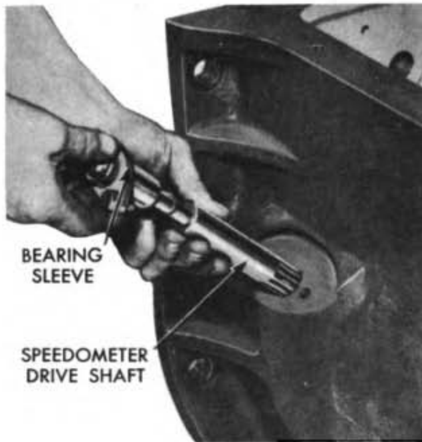
Figure 45 — Removing Speedometer Drive Shaft
