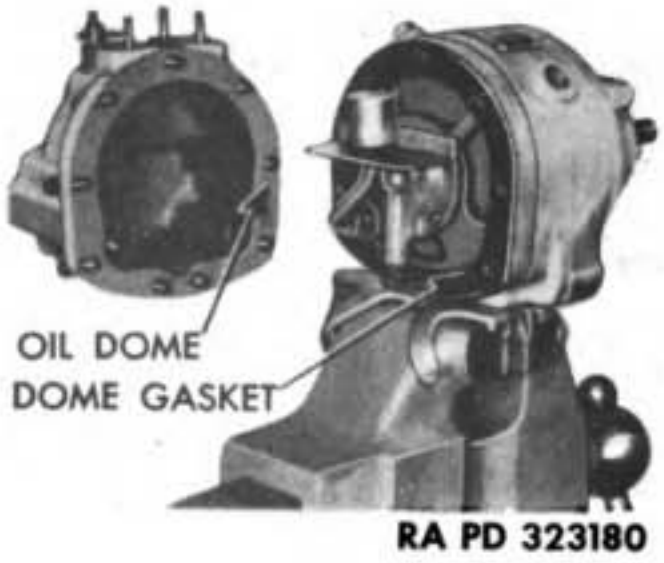
Figure 184 — Removing Oil Dome
