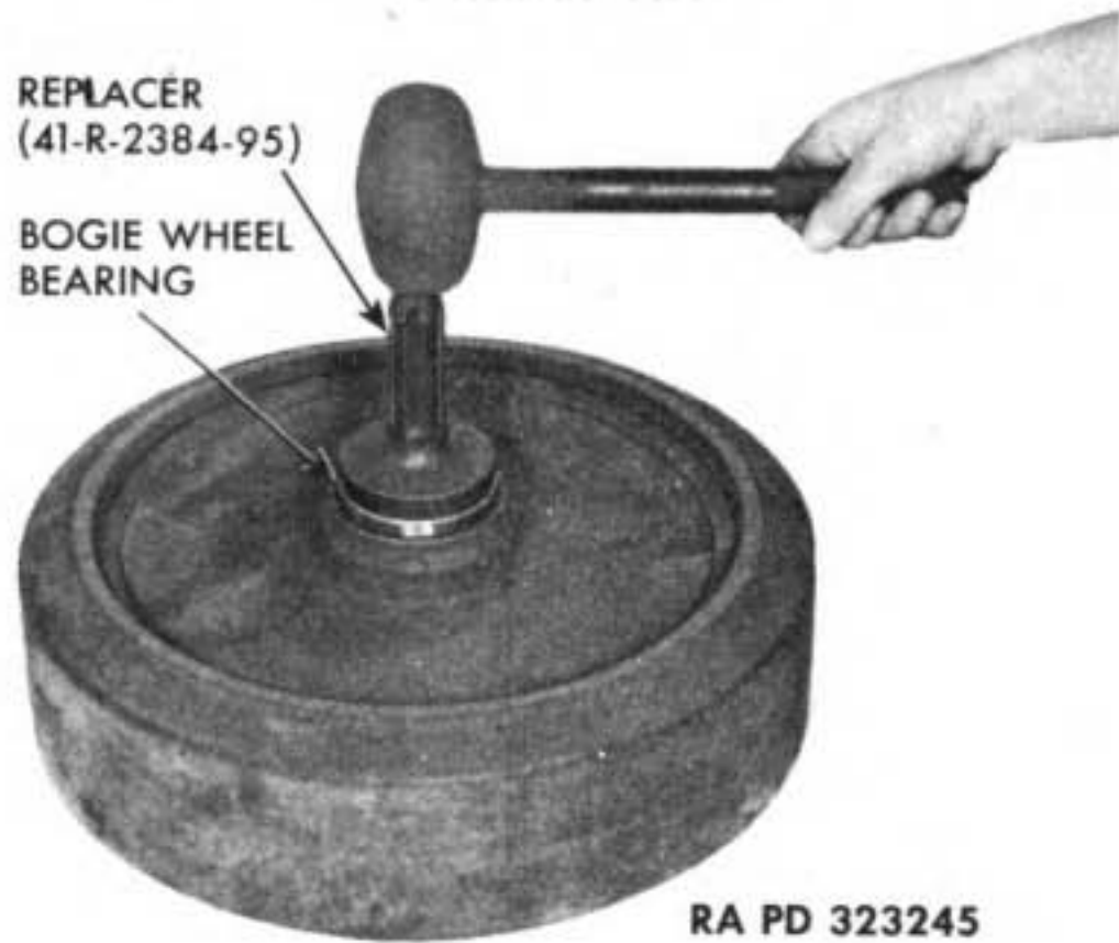
Figure 251 — Installing Bogie Wheel Bearing
