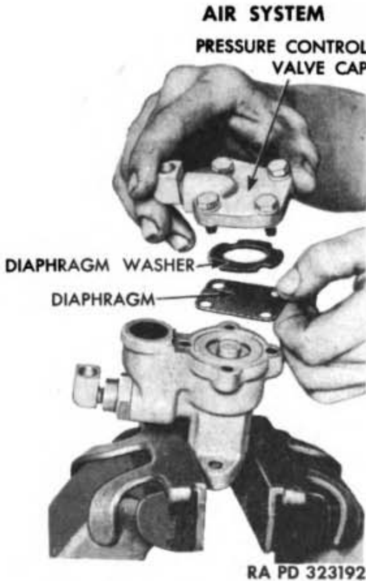
Figure 196 — Removing Cap and Diaphragm from Pressure Control Valve
