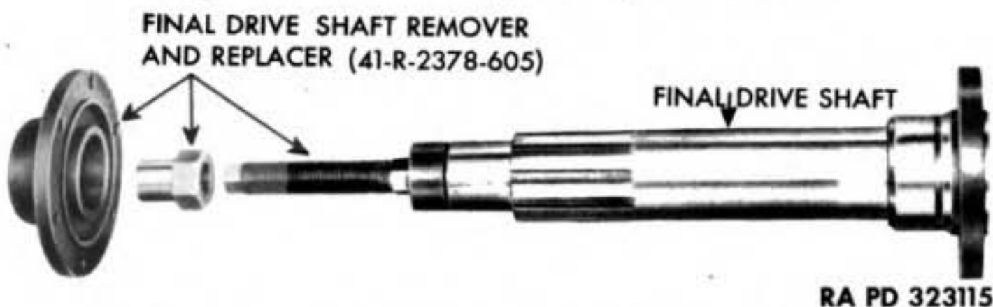
Figure 116 — Use of Tool for Removing Final Drive Shaft
