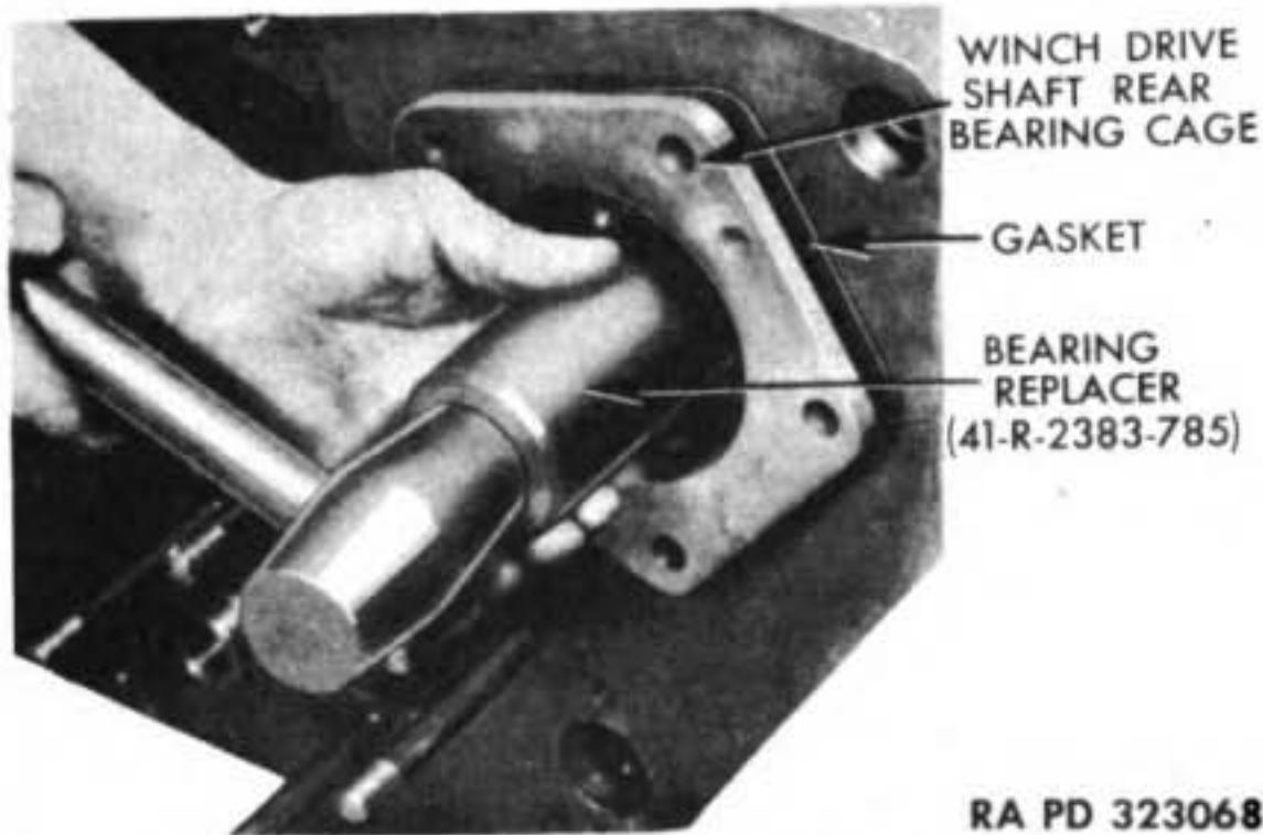
Figure 68 — Installing Winch Drive Shaft Rear Bearing and Bearing Cage
