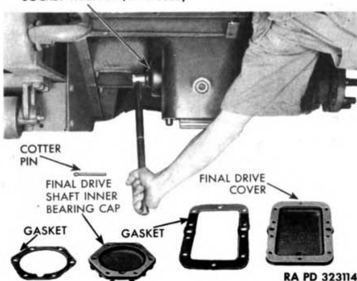
Figure 115 — Removing Bearing Retainer Nut
