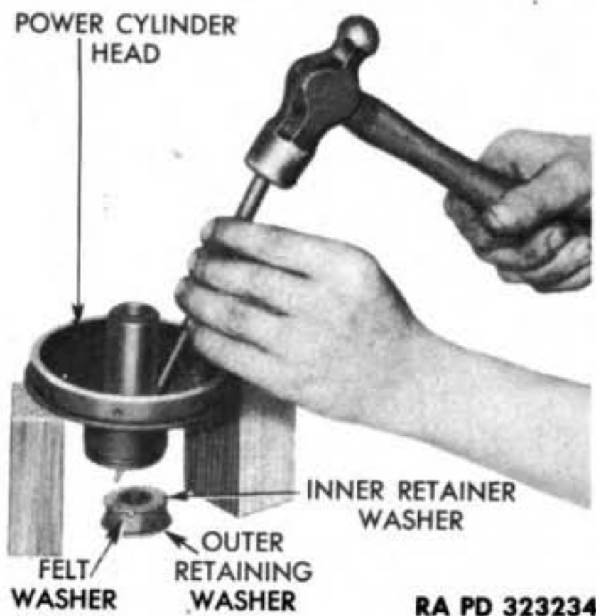
Figure 239 — Removing Washers from Power Cylinder
