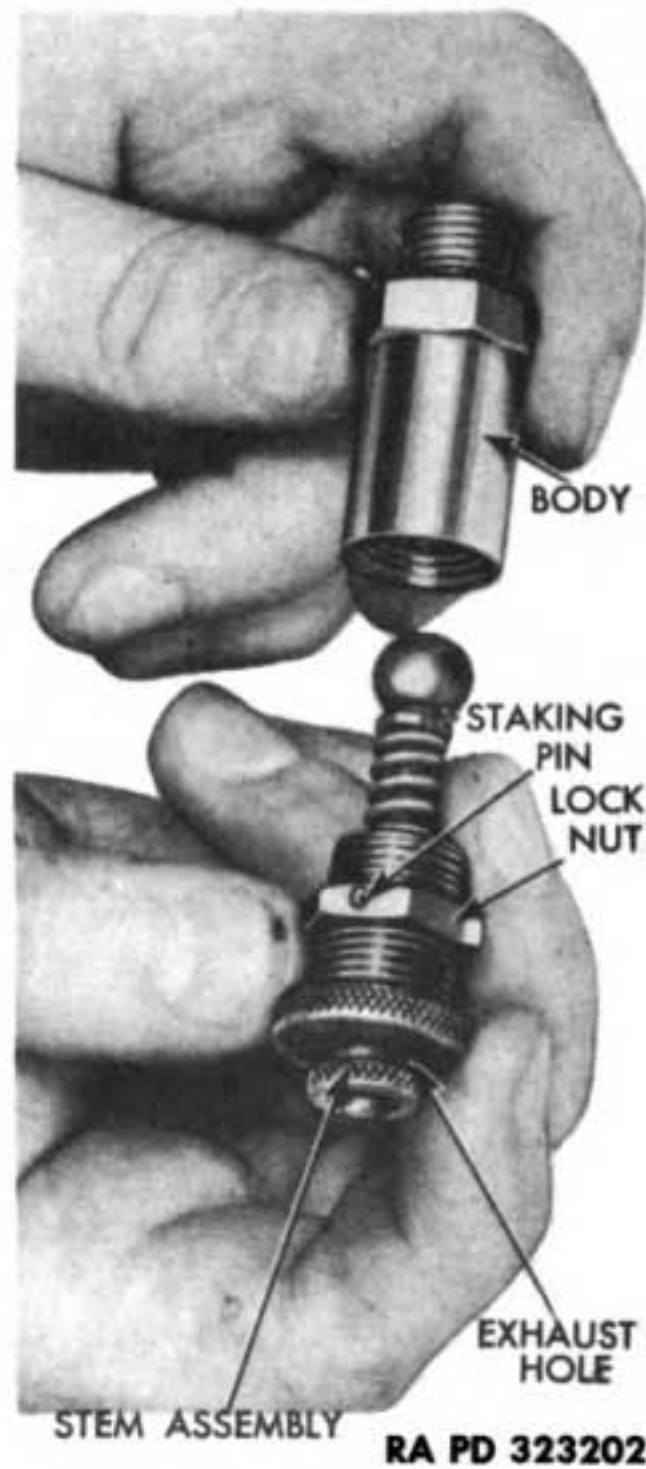
Figure 206 — Safety Valve Stem Assembly Removed from Body
