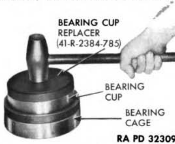
Figure 92 — Installing Differential Bearing Cup
