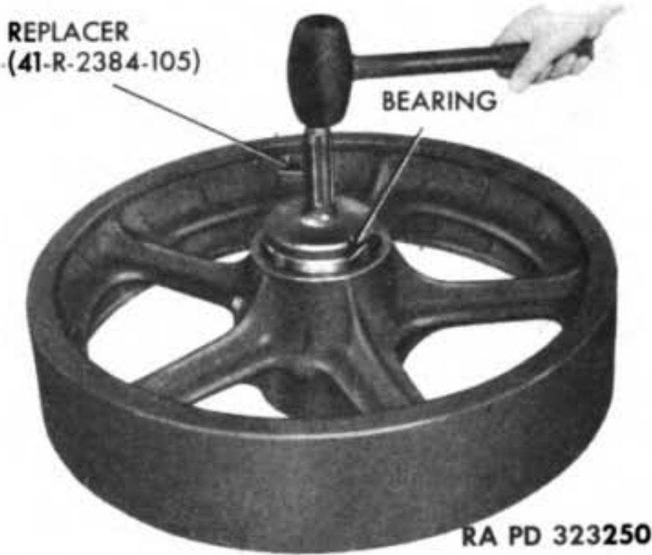
Figure 256 — Installing Trailing Idler Wheel Bearing
