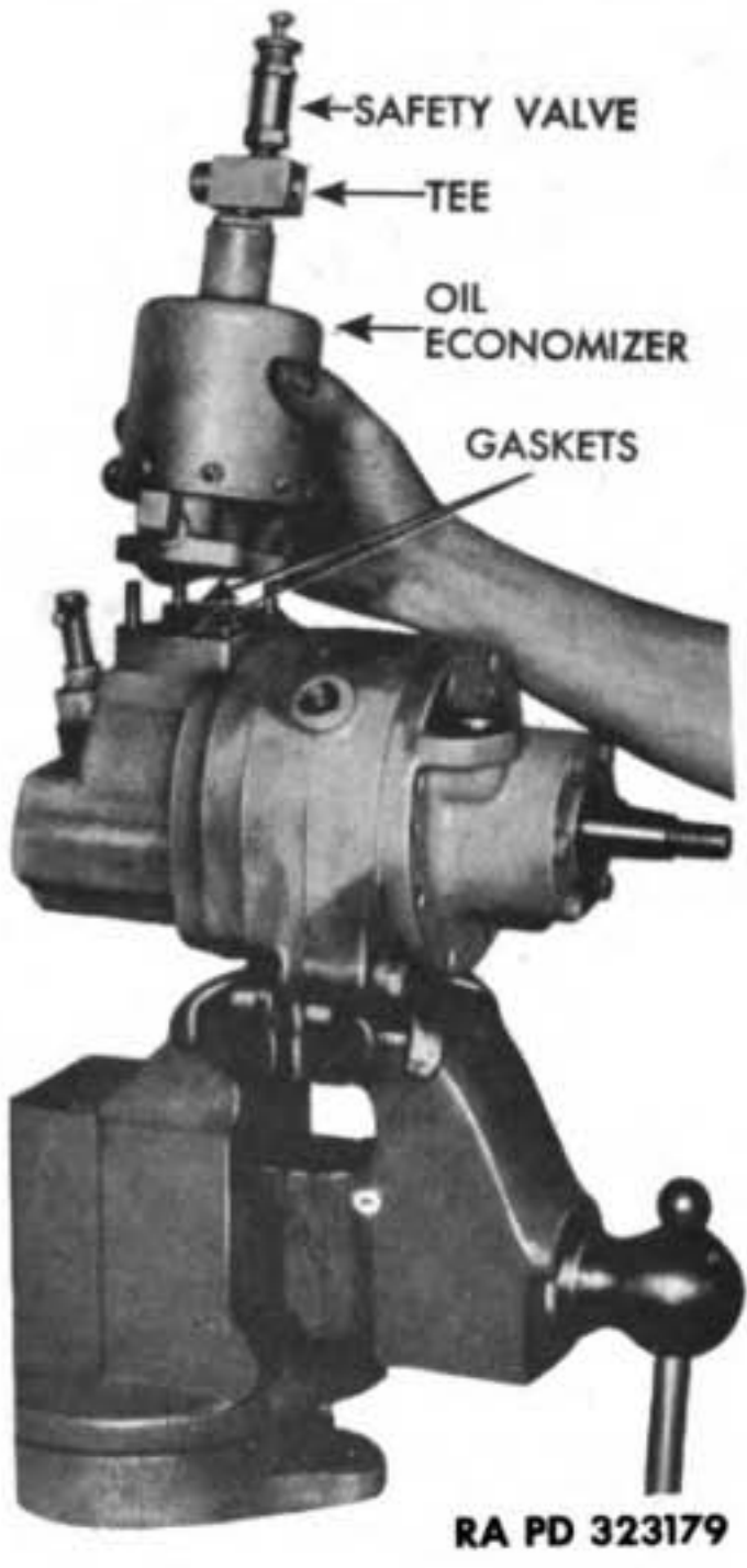
Figure 183 — Removing Oil Economizer with Tee and Safety Valve
