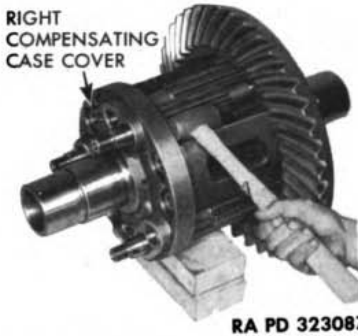
Figure 88 — Removing Right Compensating Case Cover
