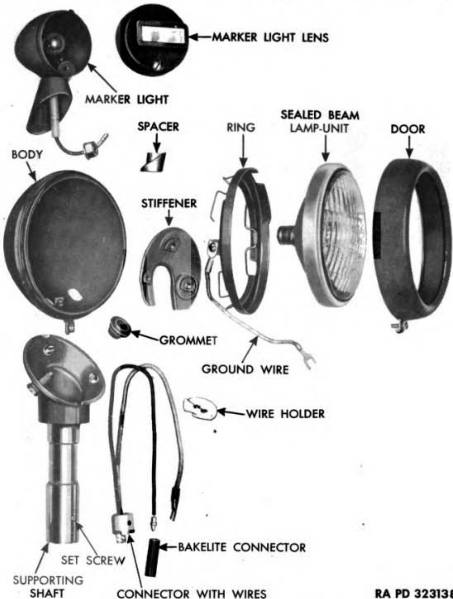
Figure 139 — Headlight Disassembled
