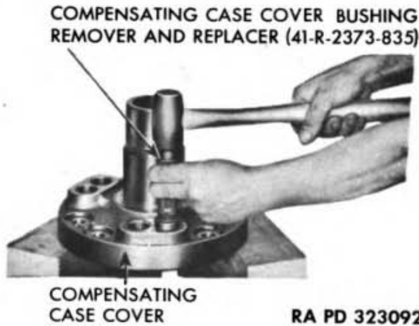
Figure 93 — Removing Compensating Case Cover Internal Pinion Bushing
