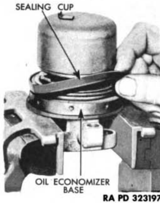
Figure 201 — Removing Sealing Cup from Oil Economizer Base
