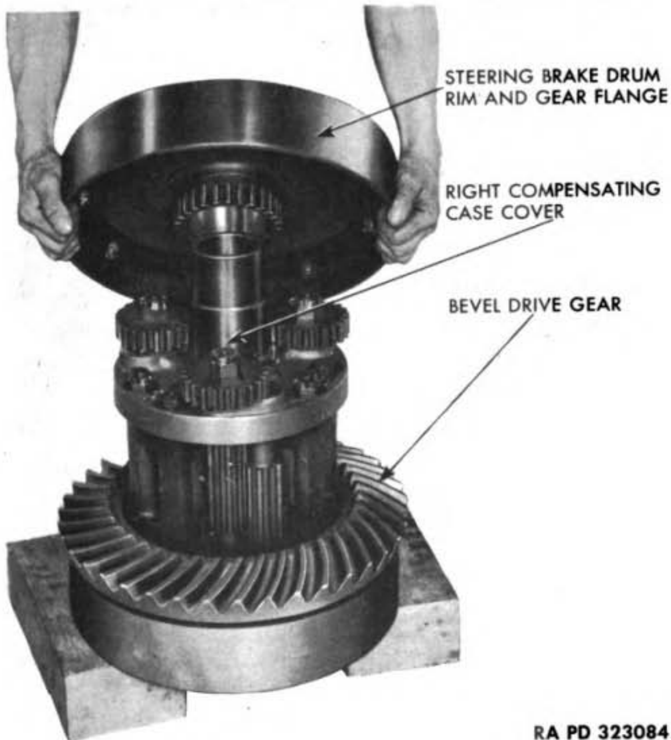
Figure 84 — Removing Steering Brake Drum Rim and Gear Flange
