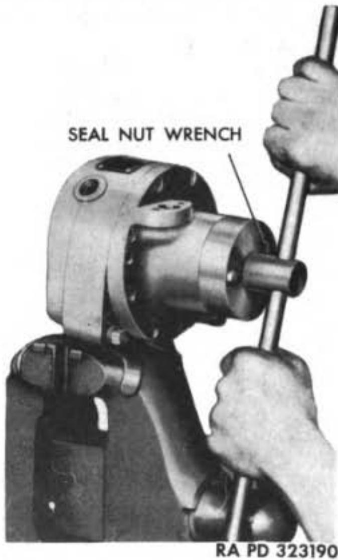
Figure 194 — Removing Sealing Nut with Wrench (41-W-3336-690)
