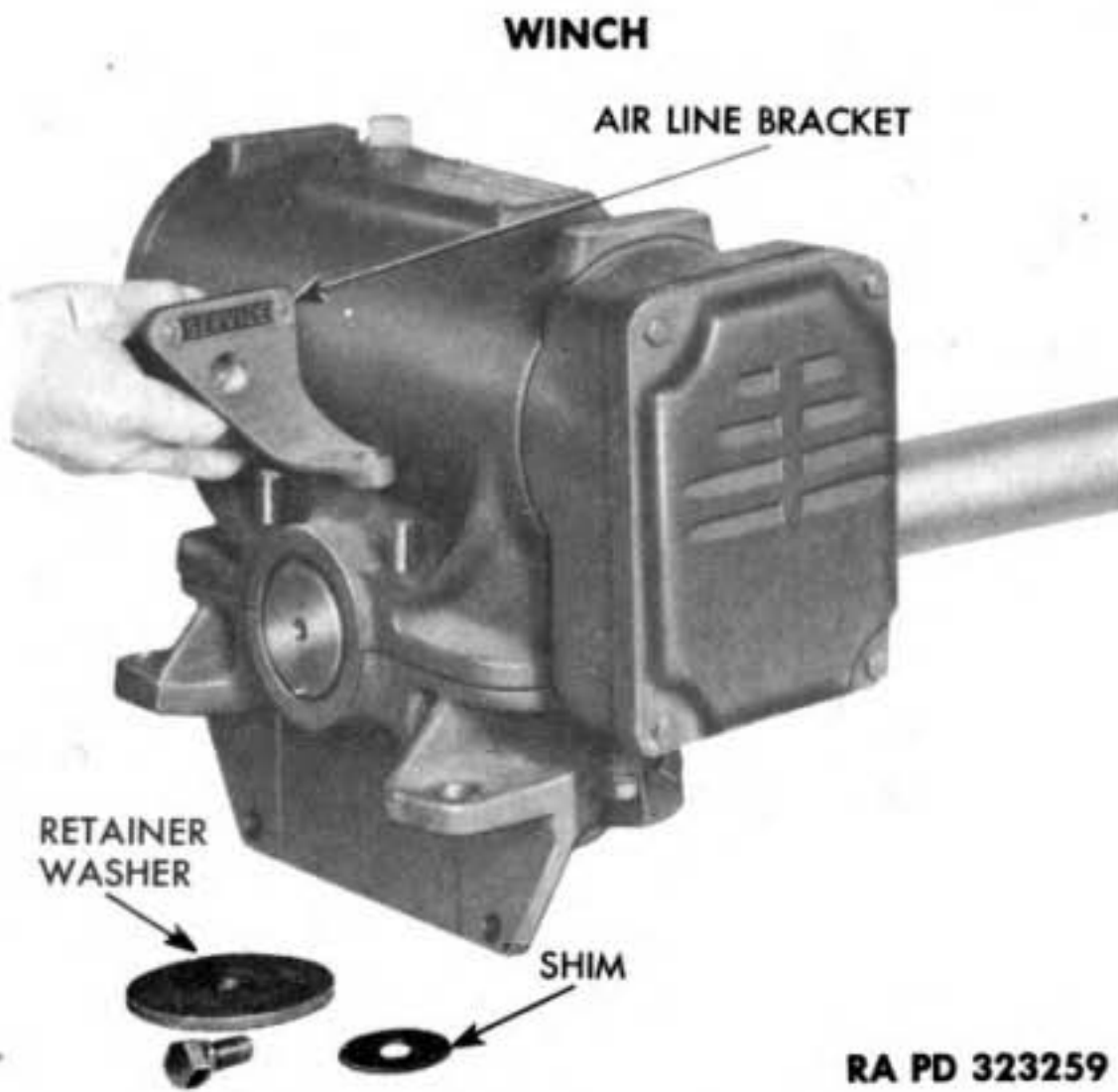
Figure 266 — Removing Air Line Bracket
