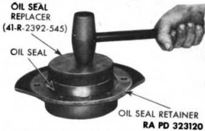
Figure 121 — Installing Final Drive Shaft Oil Seal
