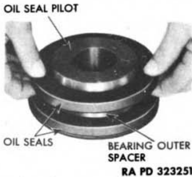
Figure 257 — Installing Oil Seals on Bearing Outer Spacer with Pilot (41-C-2562-460)
