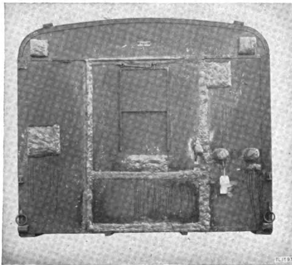
Figure 22. Shelter HO-17-A, sealing compound in place.
