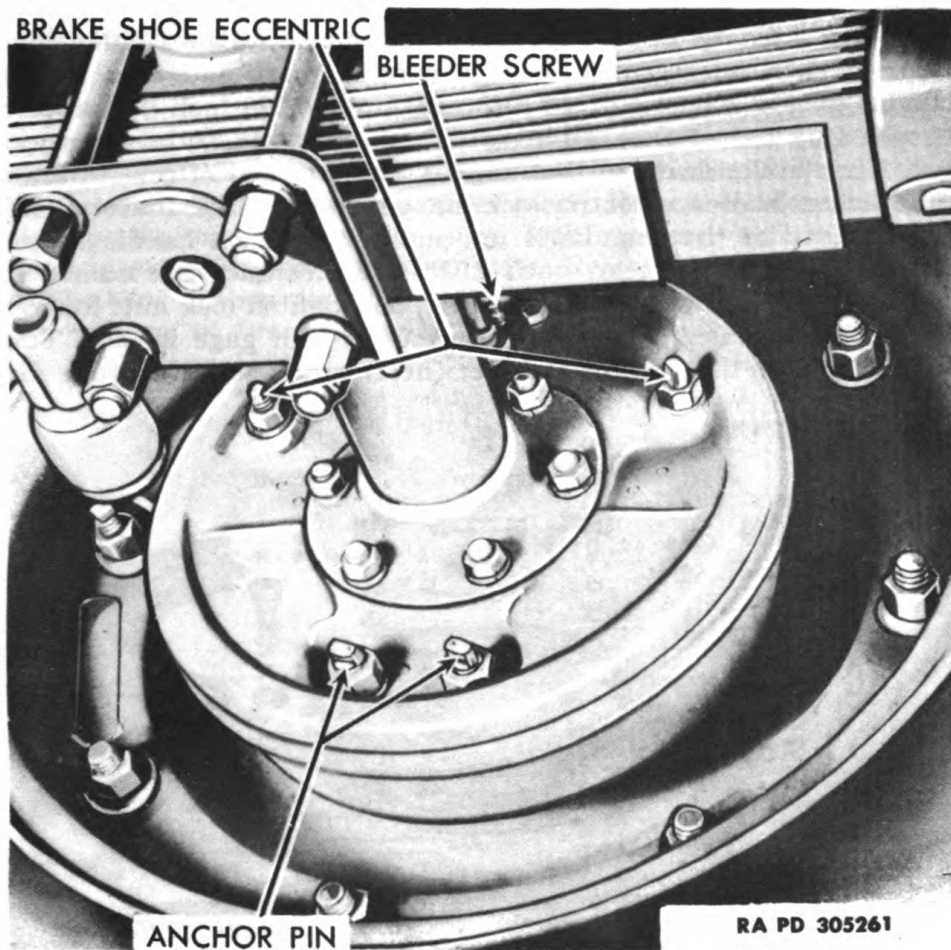
Figure 86—Wheel Brake Adjustment Points
