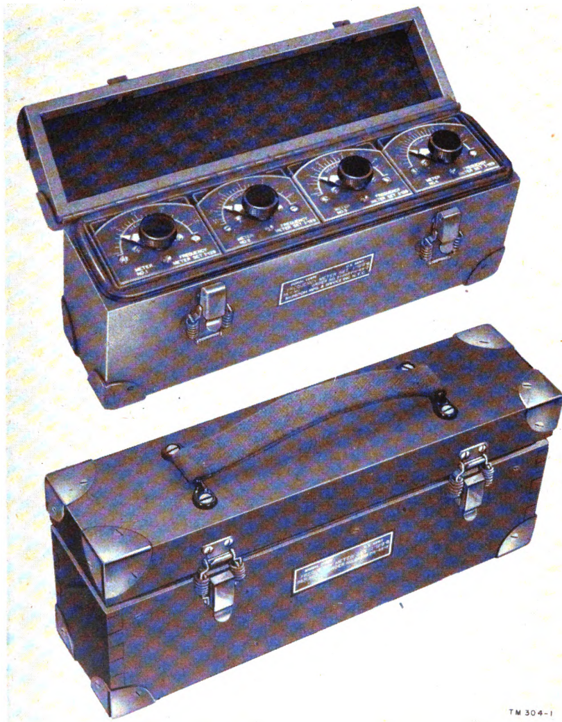
Figure 1. Frequency Meter Set I-129-B (24665-P-49), case cover open and closed.
