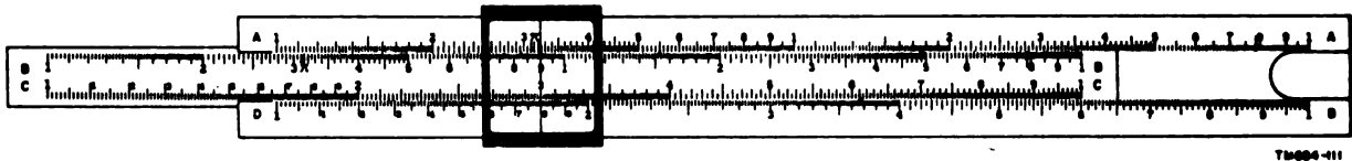
Figure 98. Slide rule arranged for multiplying 6 by 3.
