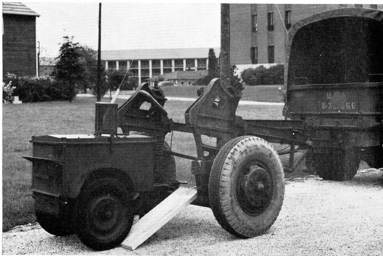
TRAILER K-38 AND TRAILER K-37 LINED UP PRIOR TO LOADING. THIS IS THE FIRST STEP IN THE SUGGESTED OPERATION.
