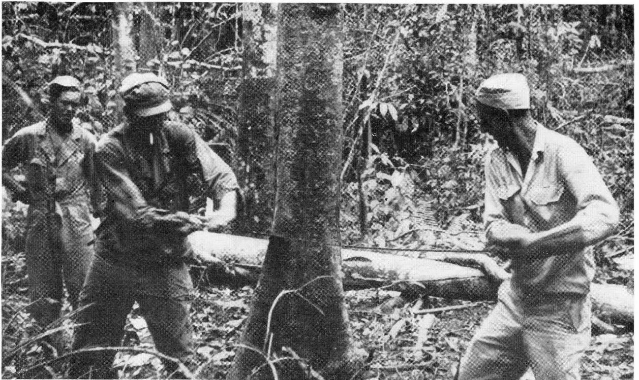
WORKING A CROSS-CUT SAW AT A SIGNAL CORPS LOGGING CAMP IN NEW GUINEA. THE NATIVES CALL THIS TOOL THE "YOU-PULLEM-YOU-PUSHEM-BIG BROTHER-OF-AX."
