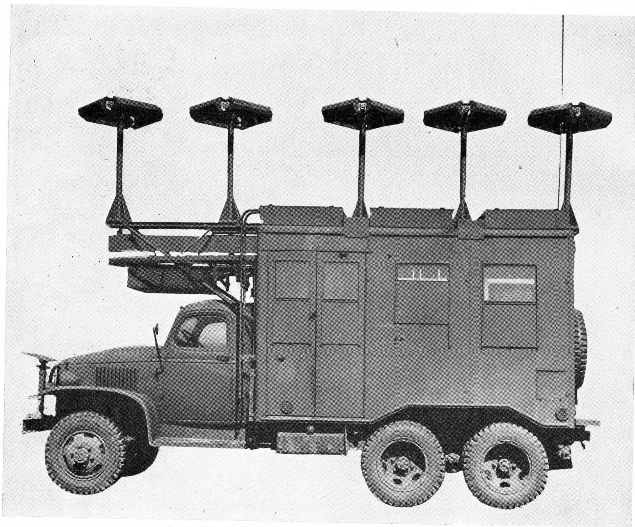
RADIO SET AN/MRN-1 LOCALIZER TRANSMITTER IN OPERATION.
