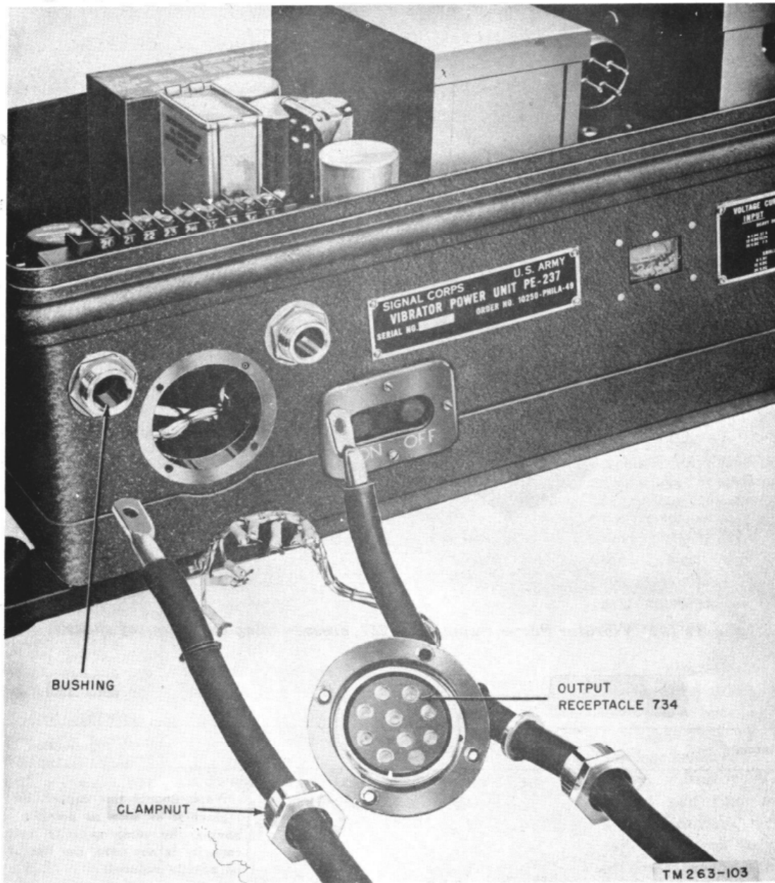
Figure 131. Vibrator Power Supply PE-237, battery cables and power output receptacle 734.
