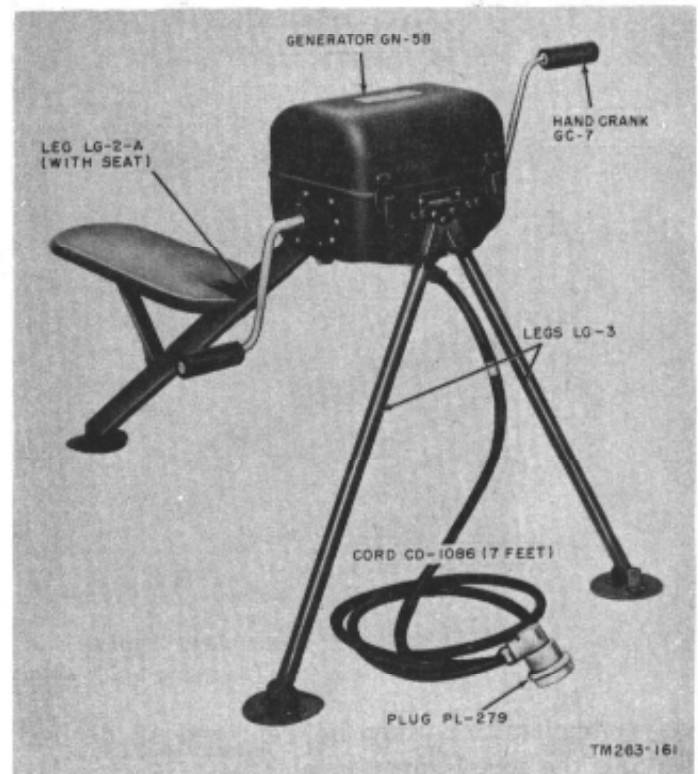
Figure 33. Generator GN-58 set up for operation.
