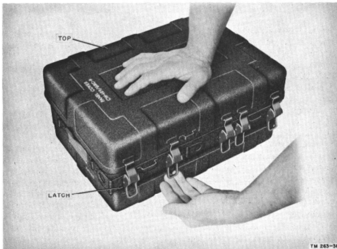
Figure 28. Removing front cover of receiver-transmitter.
