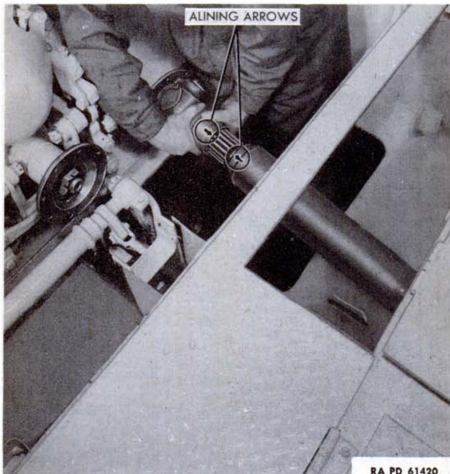
Figure 92—Removing Front Universal Joint from Propeller Shaft
