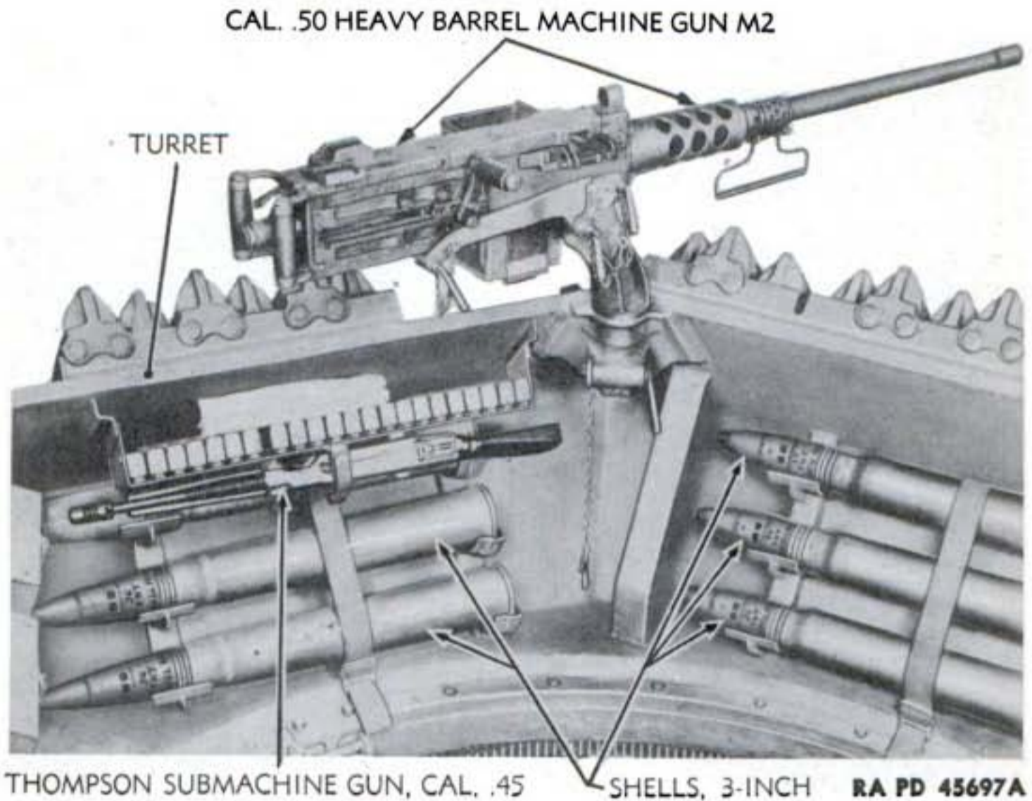
Figure 159—Rear Inside View of Turret
