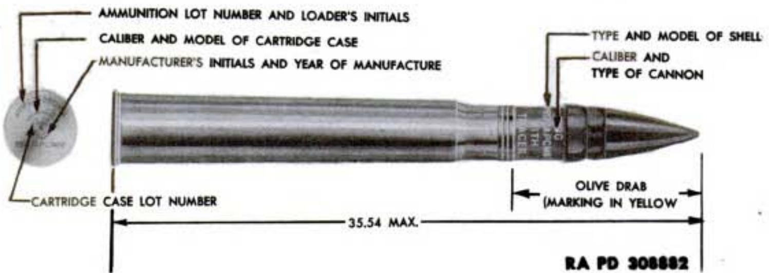
Figure 196—Projectile, Fixed, A.P.C., M62, w/Fuse, B.D., M66 or M66A1, and Tracer, 3" AA. Guns, M1918 (all models), M1, and M3, and 3" Guns, M5, M6, and M7
