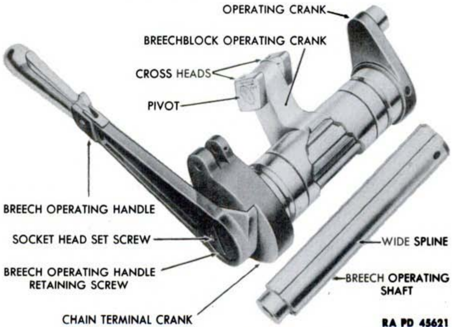
Figure 166—Breech Operating Shaft and Cranks
