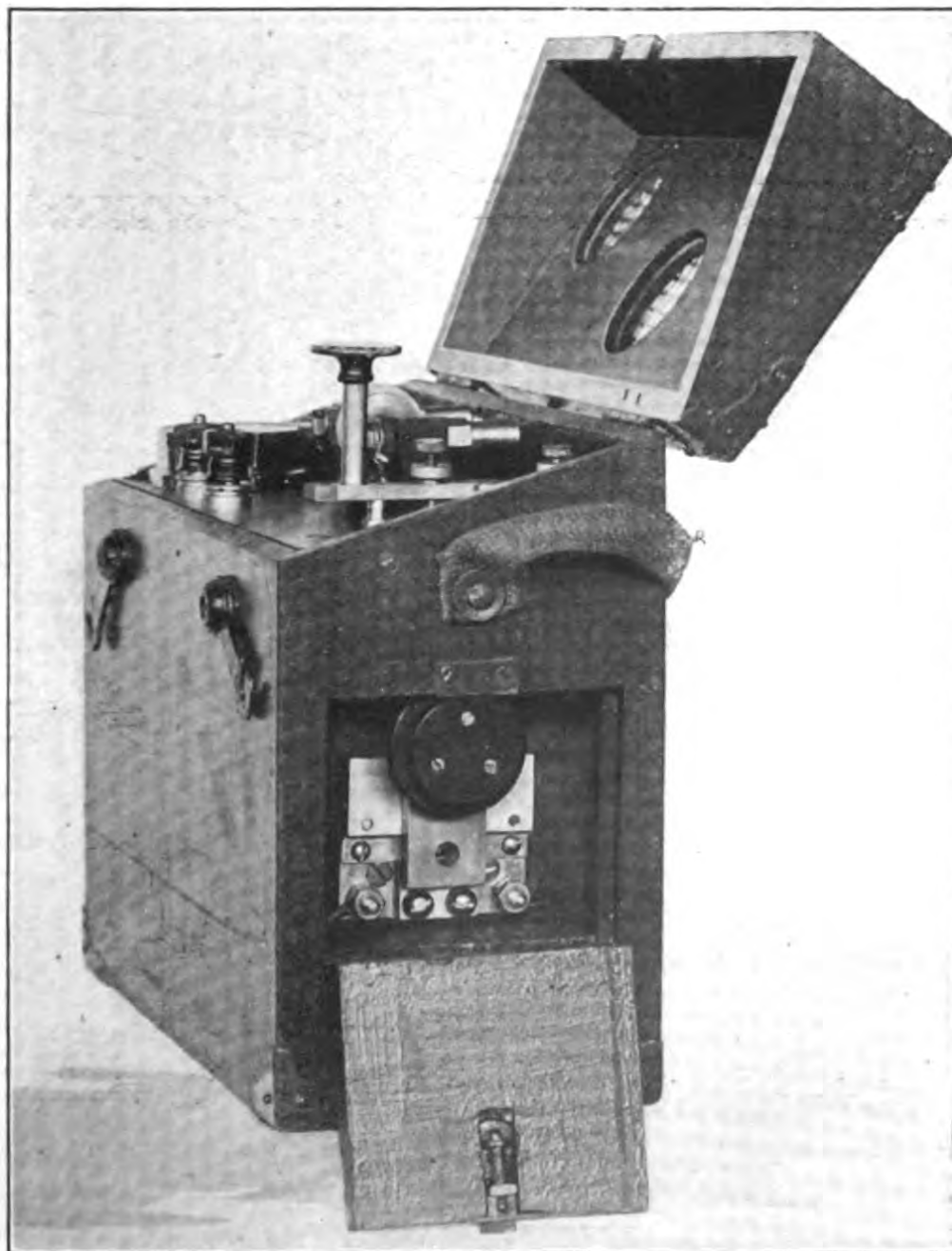
Fig. 2—Vibrator Mounted in the End of the Type BC-18 Set Box
