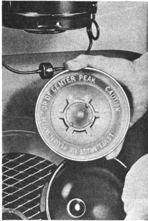
Figure 9. Putting Oil in Air Cleaner
