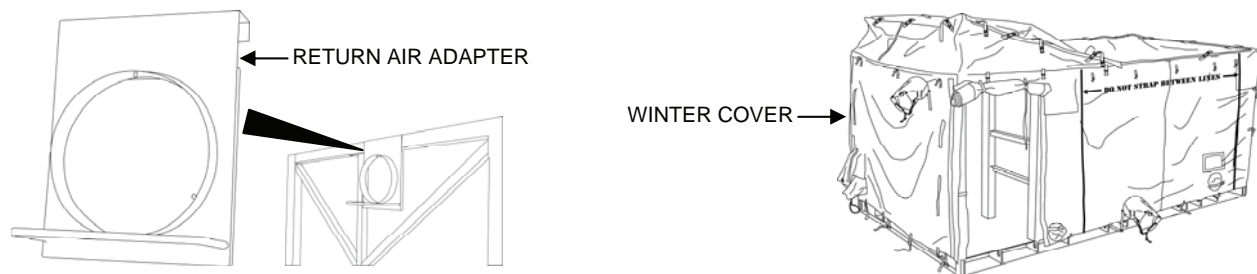
Figure 35. MC-TWPS Return Air Adapter and Winter Cover.
