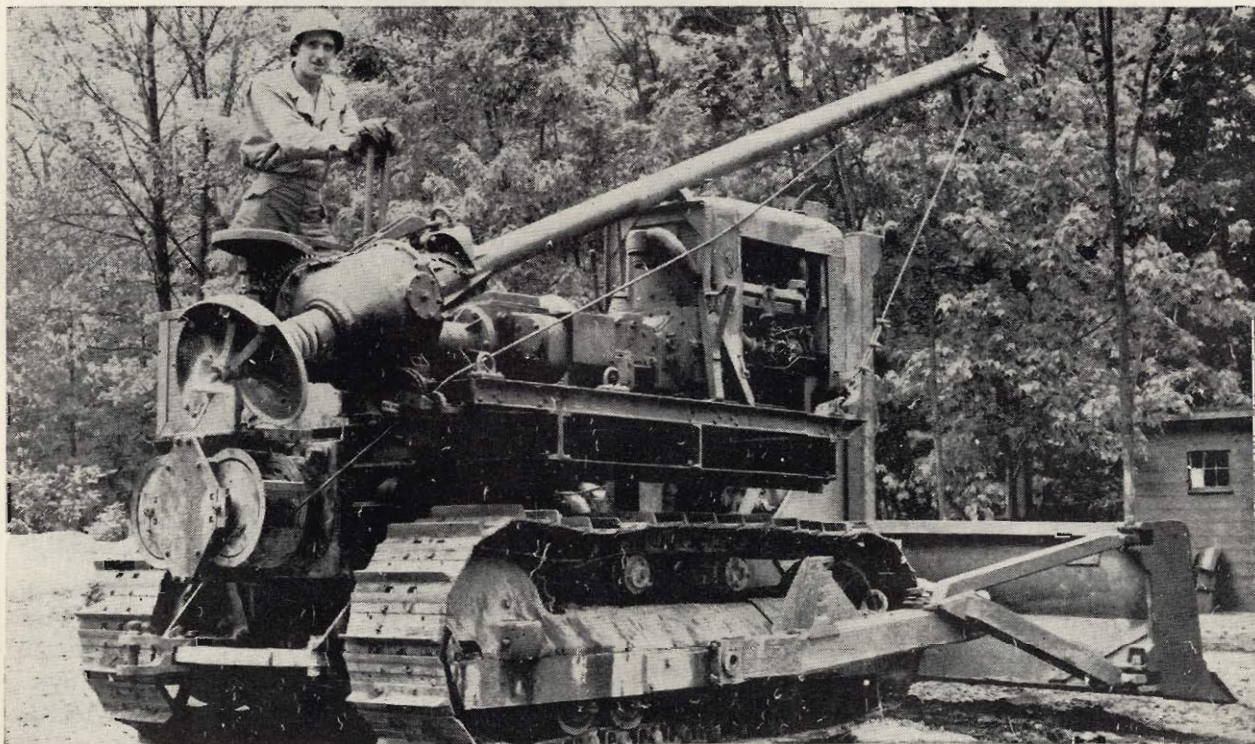
IN TRAVELING POSITION, THIS TRACTOR-MOUNTED EARTH AUGER IS JUST ABOUT TO BE PUT INTO OPERATION BY THE OPERATOR.
