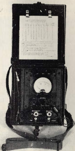
PORTABLE TEST SET FOR LINEMAN, THE TS-26/TSM.
