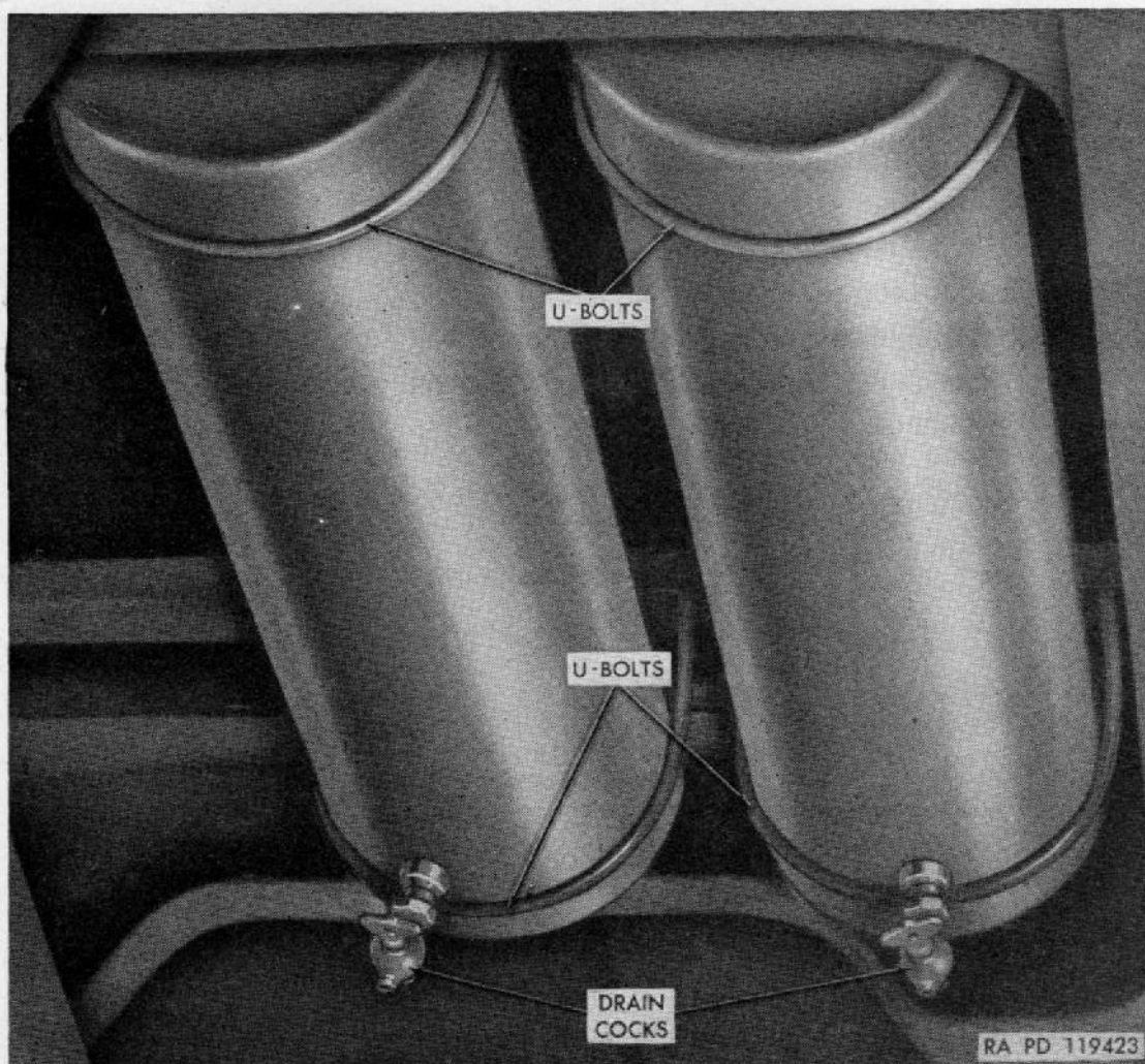
Figure 145. Air reservoir installation—M34 and M36.
