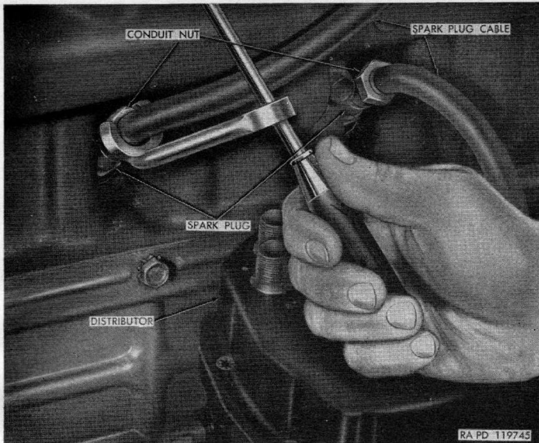
Figure 77. Using spark-plug cable conduit nut wrench 41-W-3297-760.
