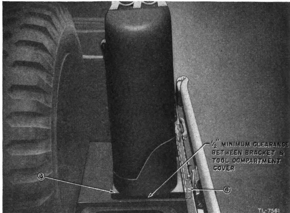
FIGURE 11.5.—Installation of gasoline container and bracket.
