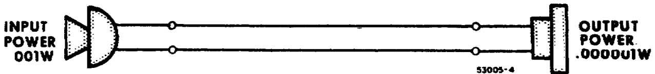
Figure 120. Circuit showing power loss.
