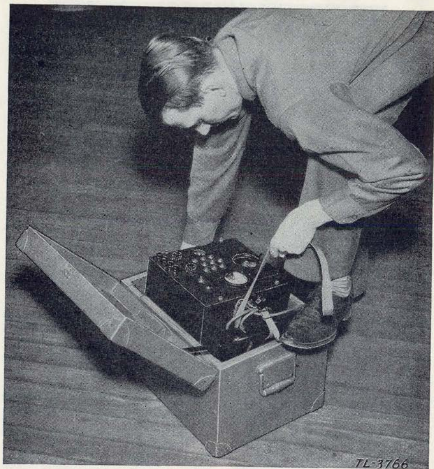
FIGURE 5.—Method of removing remote control unit RM-13-( ) from or lowering into chest CH-54-( ).
