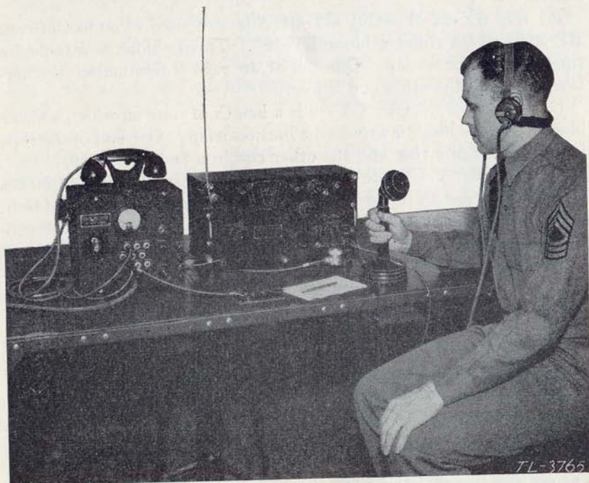
FIGURE 4.—Control unit RM-13-( ) and radio receiver BC-342-C set up to form receiving position of radio set SCR-188-A.
