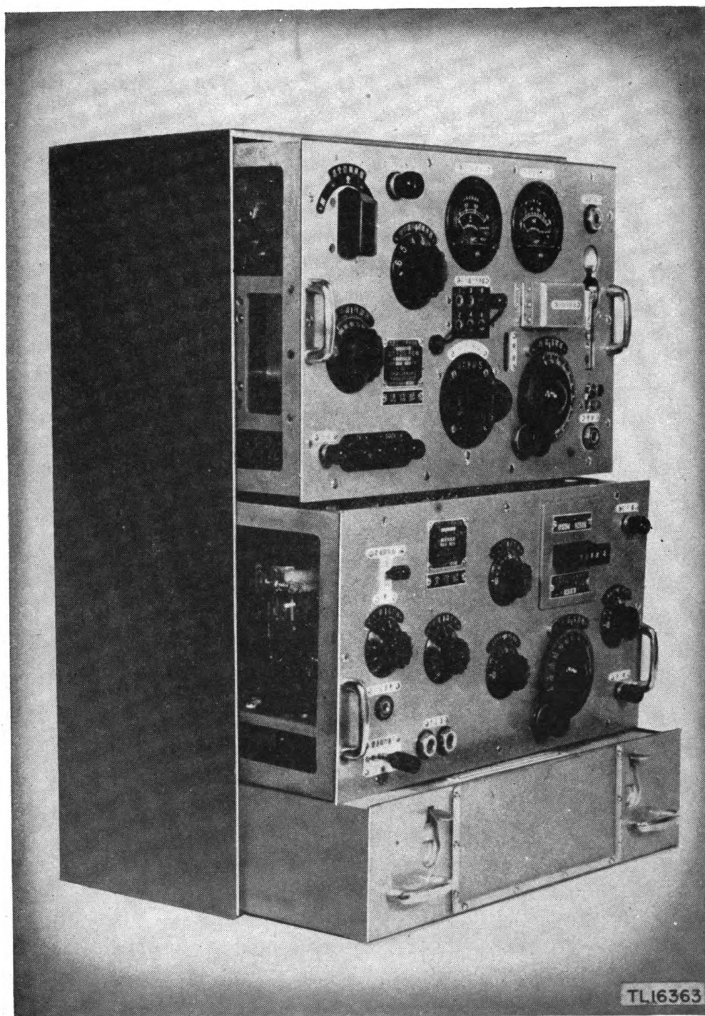
Model 94 Mark 3A Wireless Set: Mark 36 Type D Transmitter, Mark 36 Type D Receiver.
