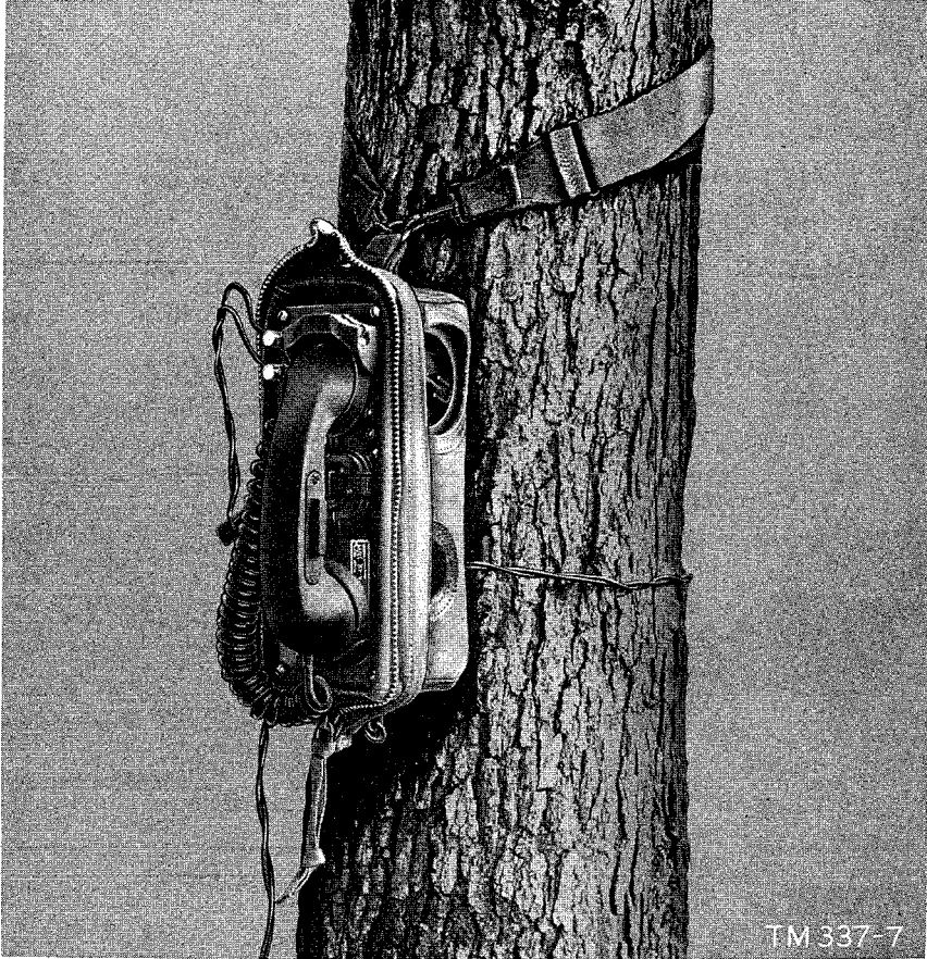
Figure 1. Telephone set TA-43/PT.
