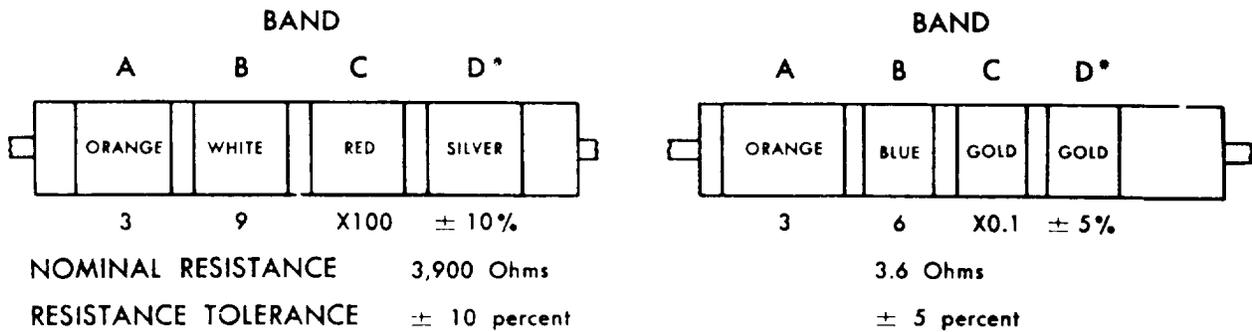
\*If Band D is omitted, the resistor tolerance is ± 20%, and the resistor is not Mil-Std.
