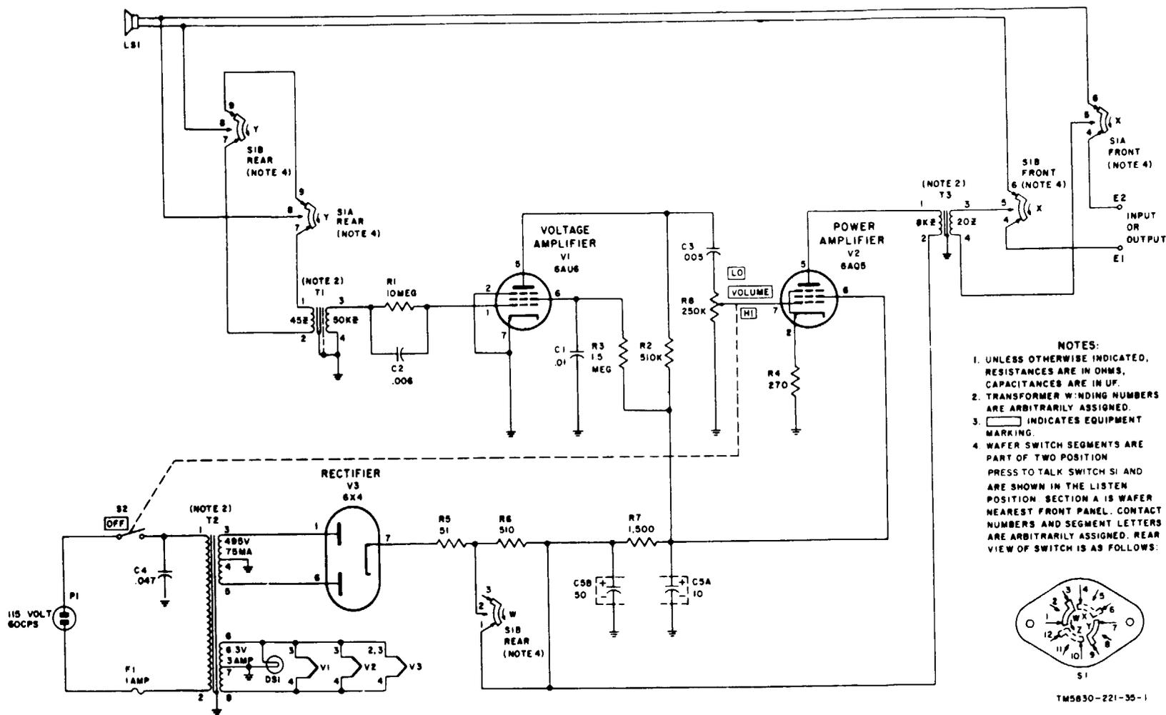
Figure 1. Intercommunication Station LS-147A/FI or LS-147B/FI, schematic diagram.
