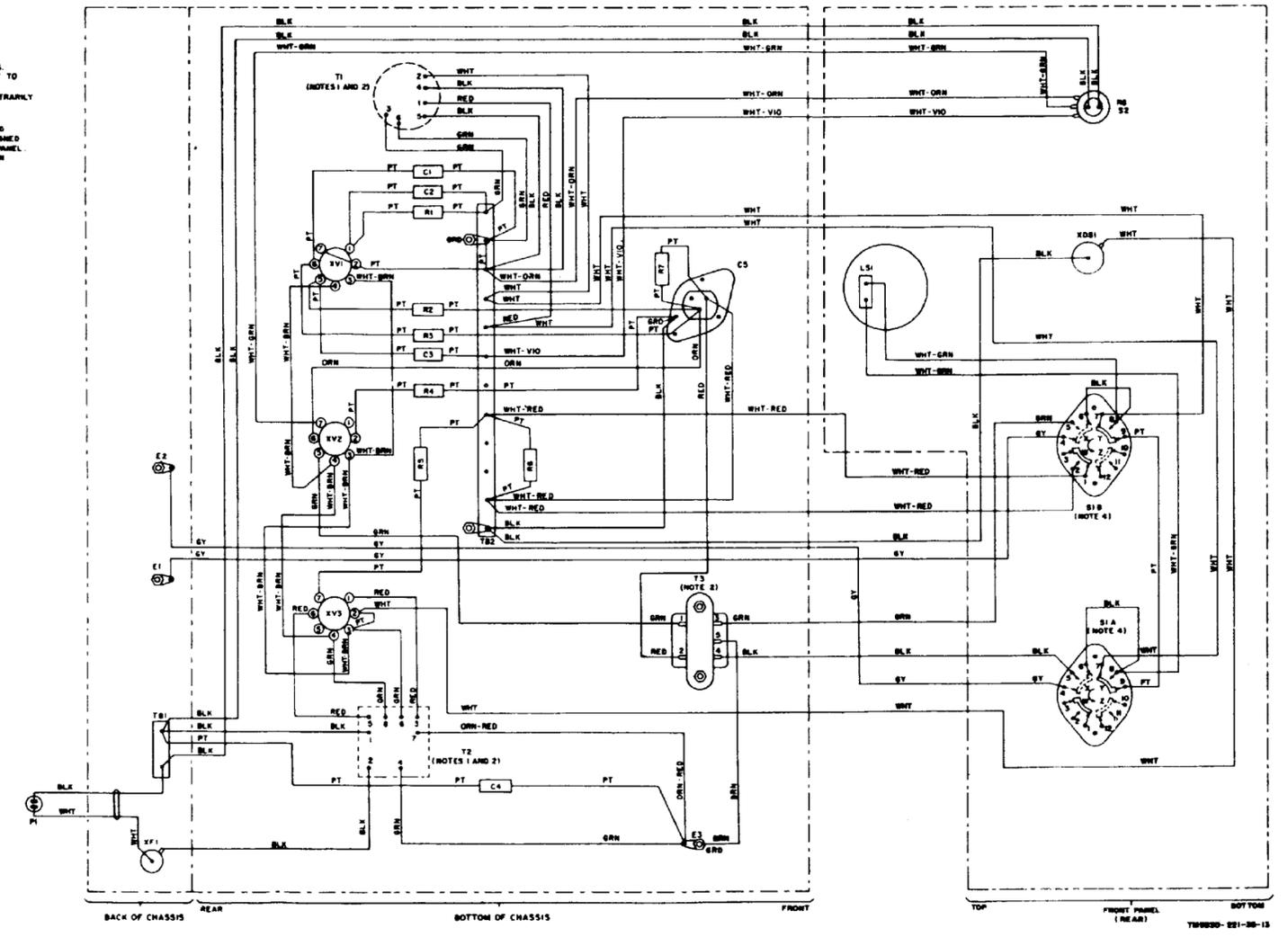
Figure 16. LS-147A/F1 or LS-147B/F1, wiring diagram.
