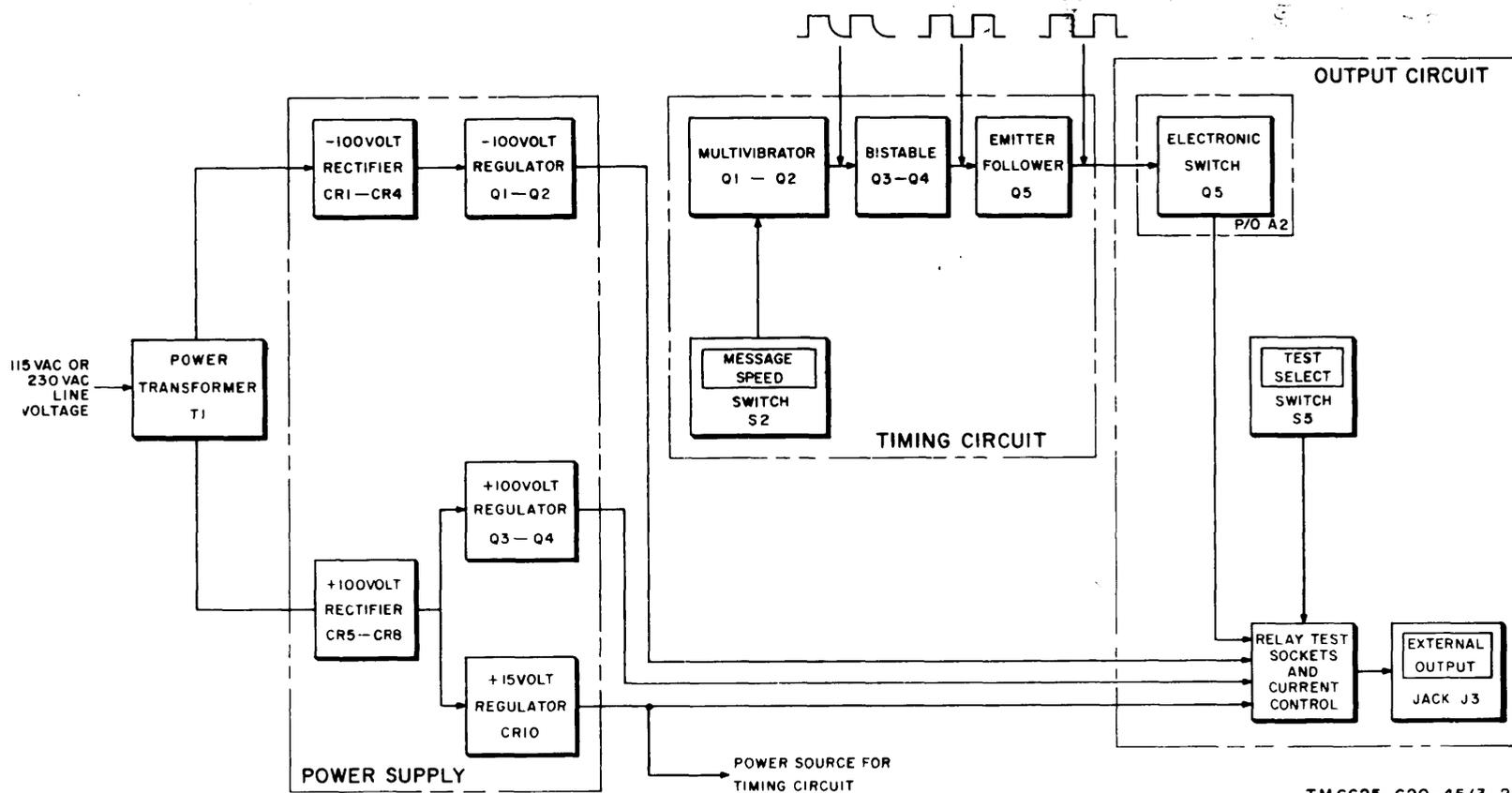
Figure 2-1. Test Set, Relay TS-836/UGM-1 block diagram.
