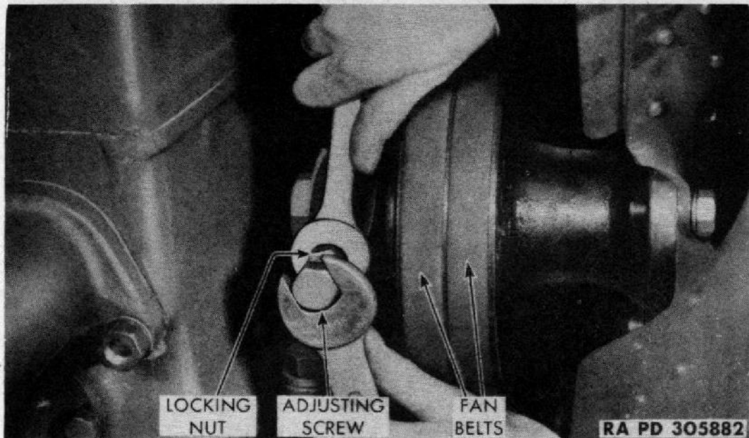
Figure 60—Adjusting Fan Belt Tension
