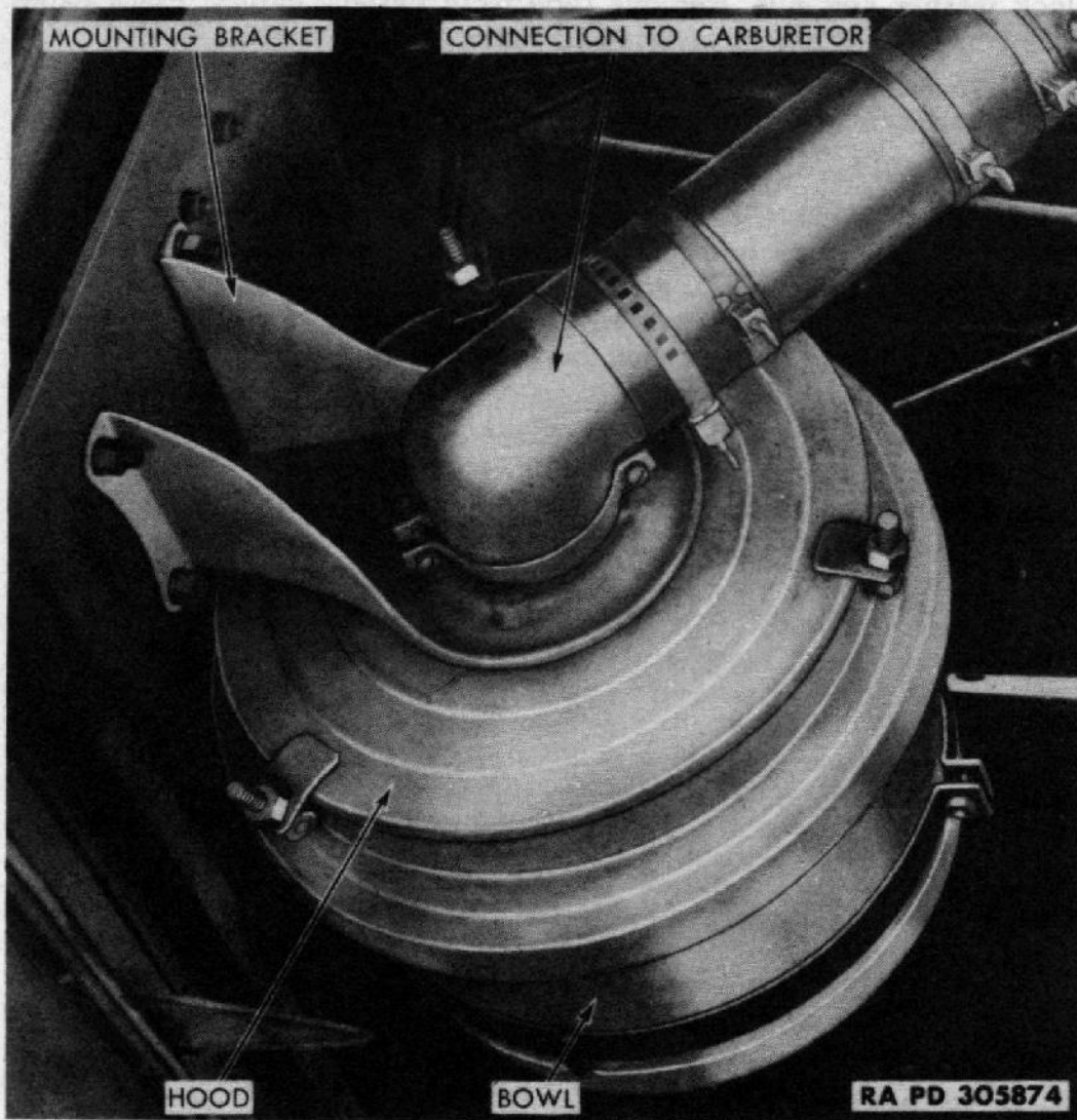
Figure 49—Air Cleaner Installed
