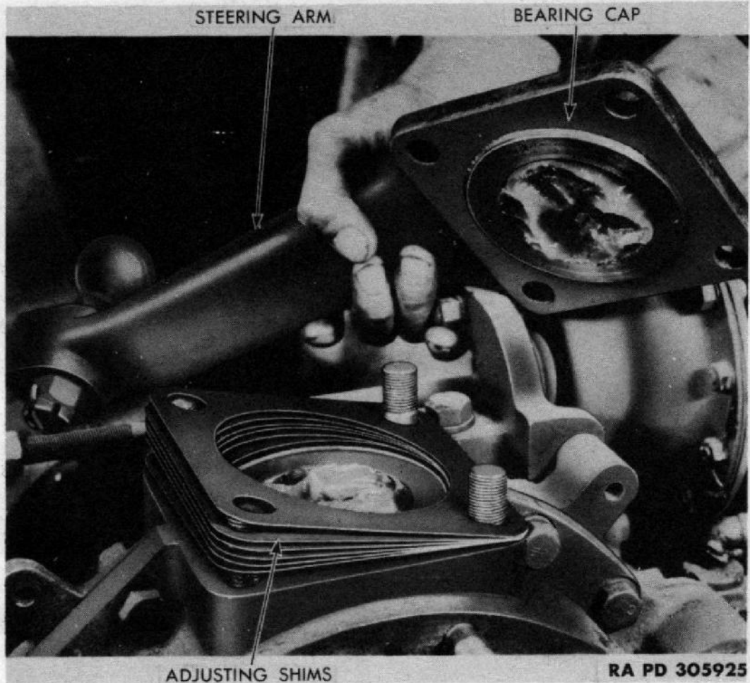
Figure 108—Removing Steering Arm and Bearing Cap Assembly
