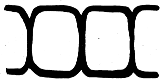
DISCRIMINATOR OUTPUT 65-CYCLE DOTS LOW-PASS FILTER OUT B
