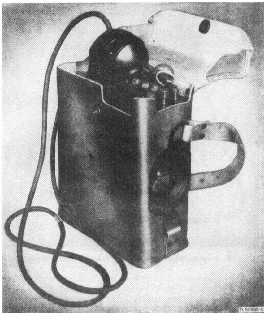
Figure 17. Telephone EE-8-B, position of handset on lever switch with case open.
