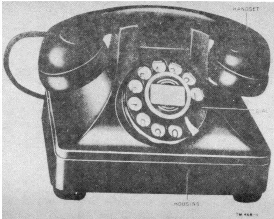
Figure 10. Telephone TP-6 (North Elec Mfg No. H-600SL), arranged for dial operation
