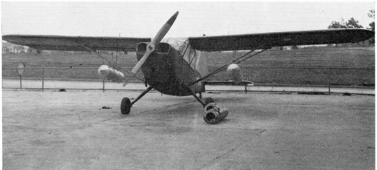
AN L-5 AIRCRAFT WITH TWO CONTAINERS, AERIAL WIRE DELIVERY, TYPE A-1, ATTACHED. THE CONTAINER AT THE RIGHT ON THE GROUND IS OPEN TO SHOW METHOD OF STOWING EIGHT WIRE DISPENSERS.
