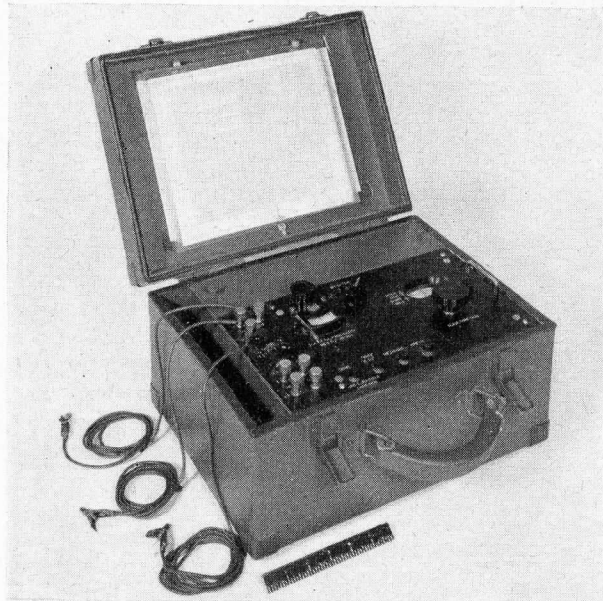
TEST SET TS-27/TSM IS USED FOR LINE TESTING WIRE AND CABLE LINES. THIS VIEW SHOWS THE PANEL ARRANGEMENT AND TABULATED DATA CHART INSIDE THE COVER.
