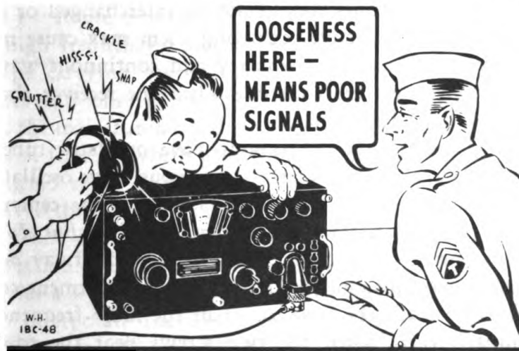
INSERT PLUGS OF THE PL-114 TYPE FULLY BEFORE YOU TIGHTEN THE KNURLED RING
