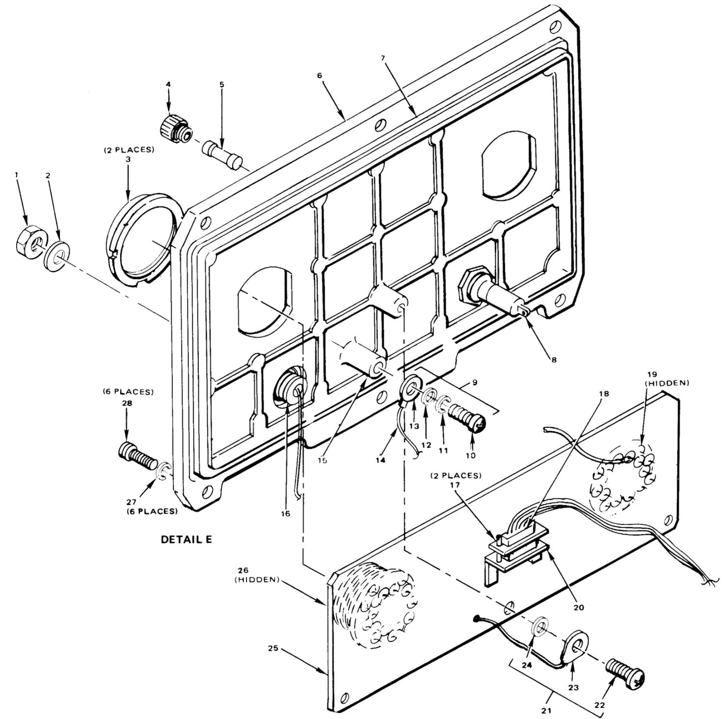
Figure 4-4. Amplifier-Converter Component Location
