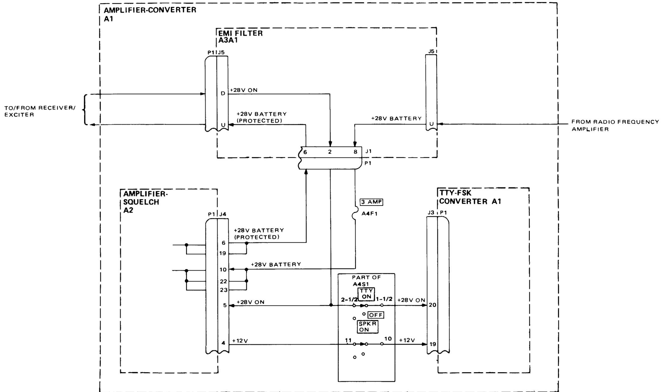
Figure 4-3. Amplifier-Converter A1 Power Distribution
