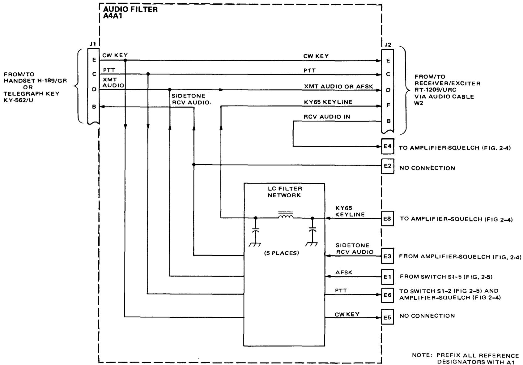
Figure 2-3. Audio Filter A1A4A1 Detailed Block Diagram
