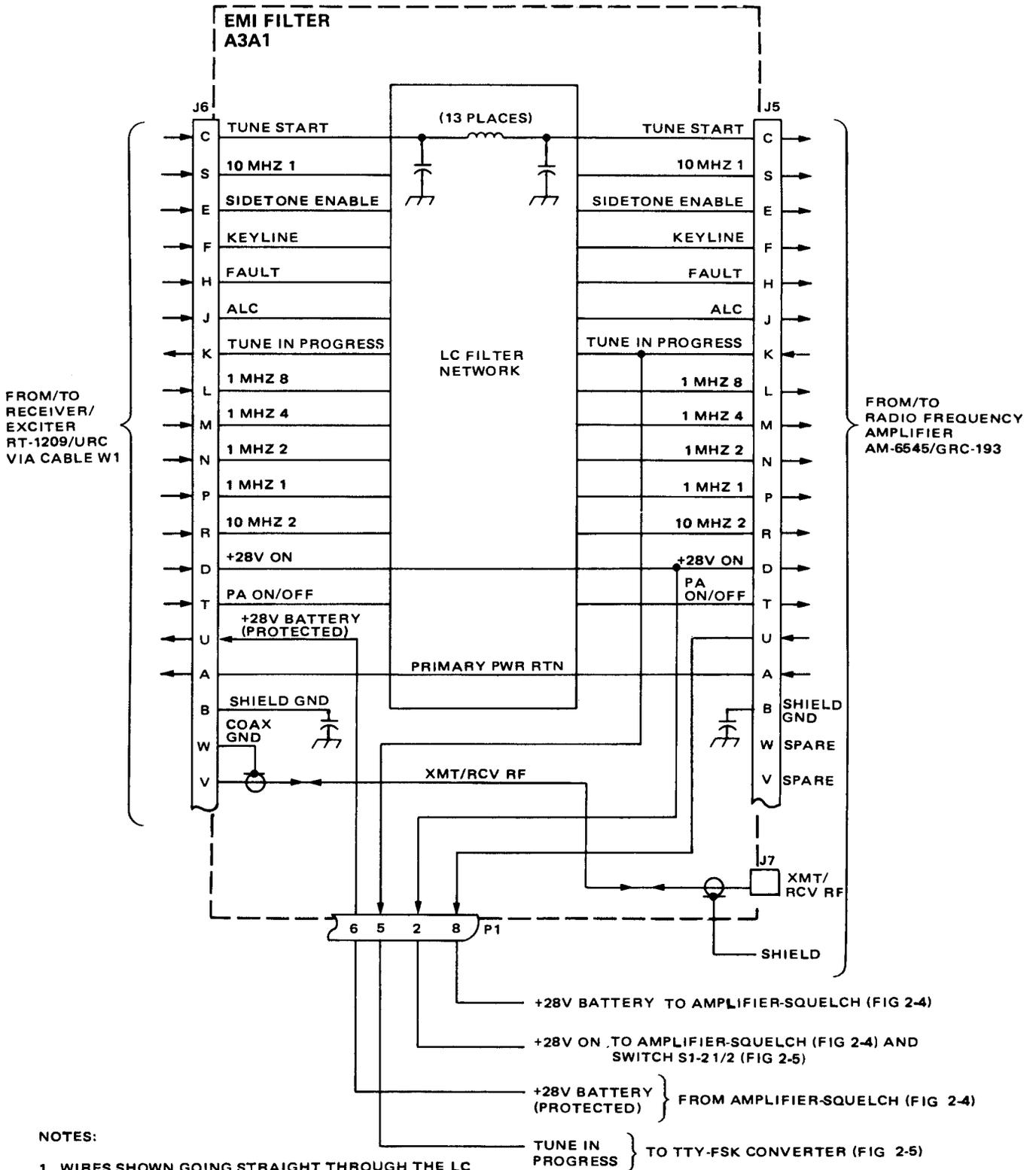
Figure 2-2. EMI Filter A1A3A1 Detailed Block Diagram
