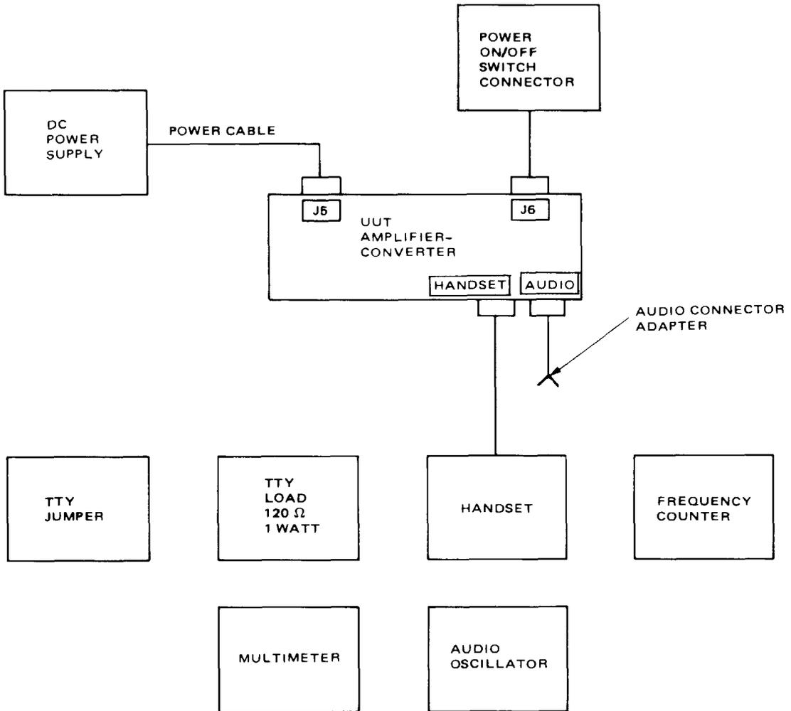
Figure 4-6. Amplifier-Converter A1 Test Setup
