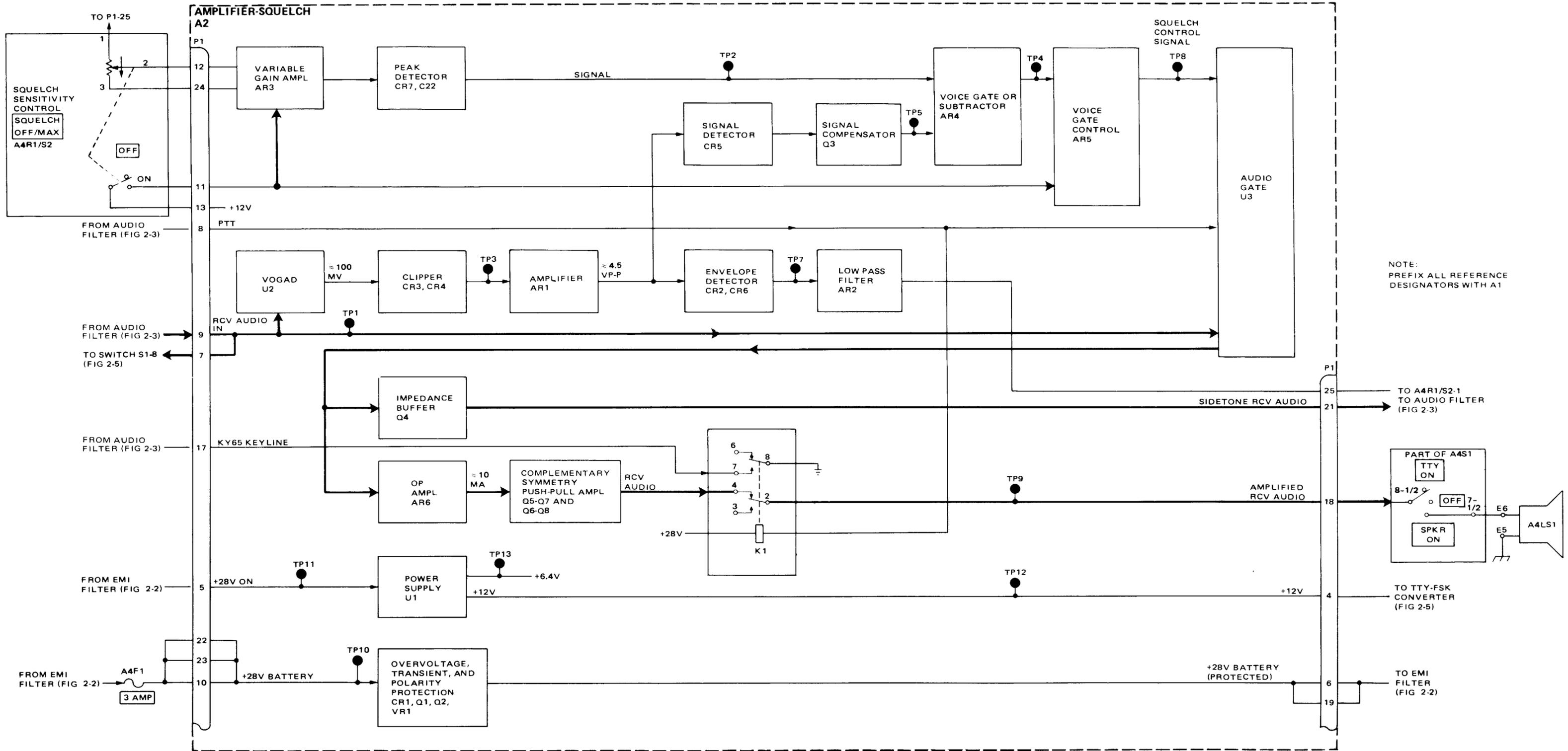
Figure 2-4. Amplifier-Squelch A1A2 Detailed Block Diagram
