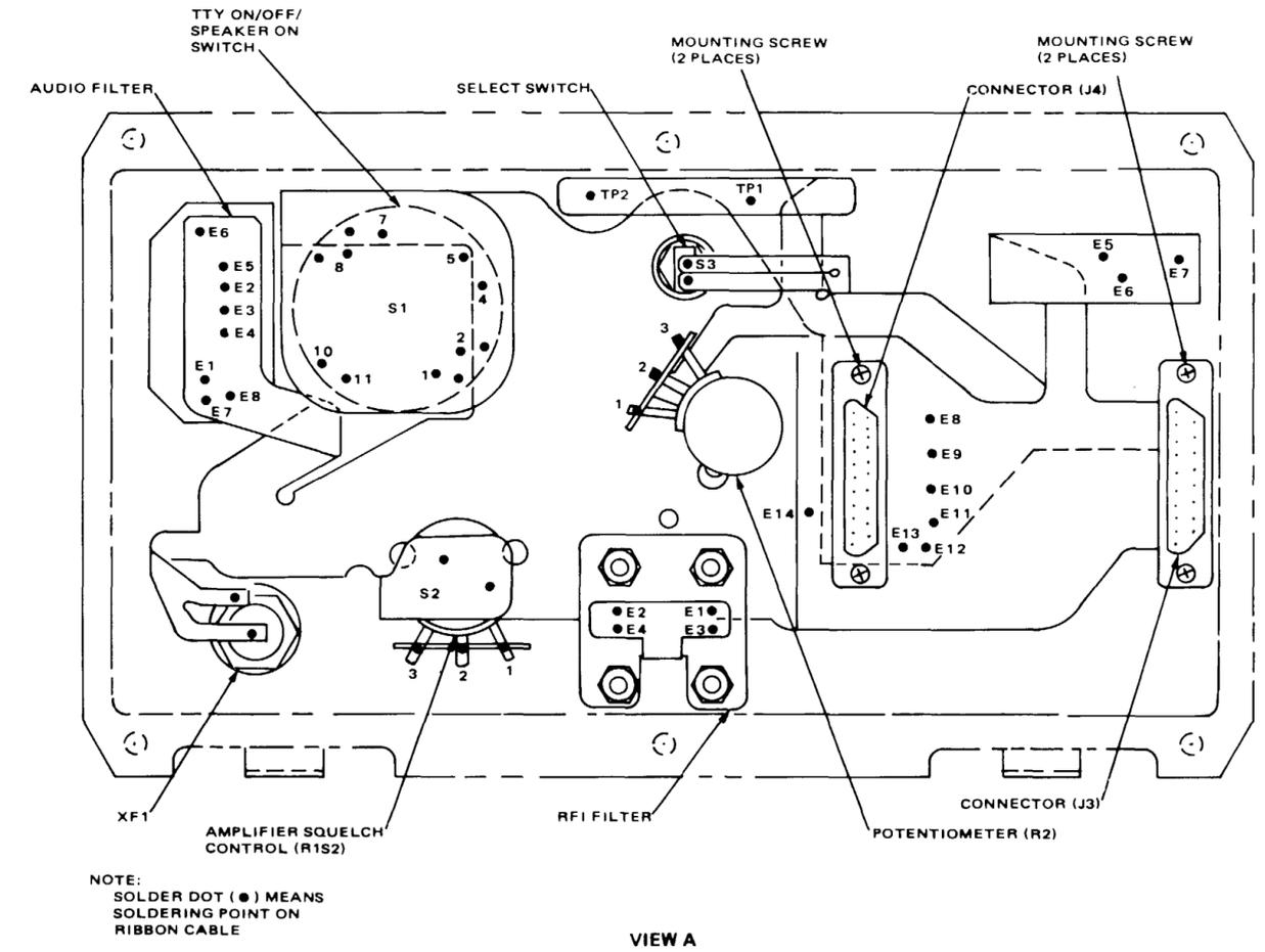
Figure 4-5. Amplifier-Converter Component Location
