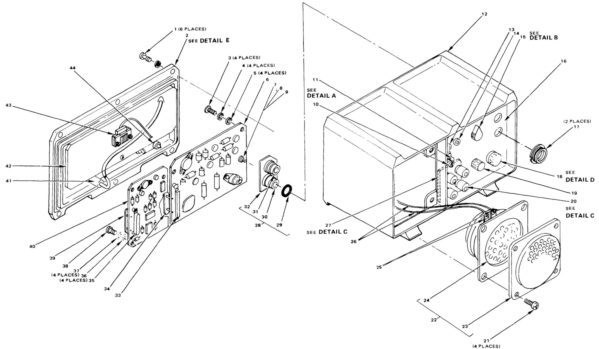
Figure 4-4. Amplifier-Converter Component Location
