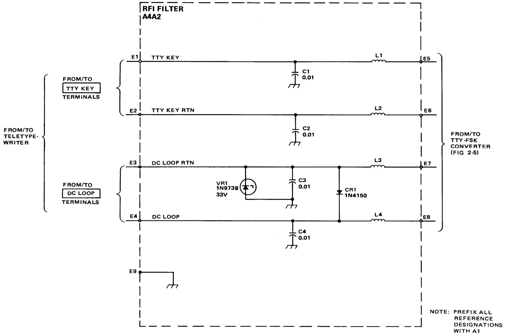
Figure 2-6. RFI Filter A1A4A2 Detailed Block Diagram
