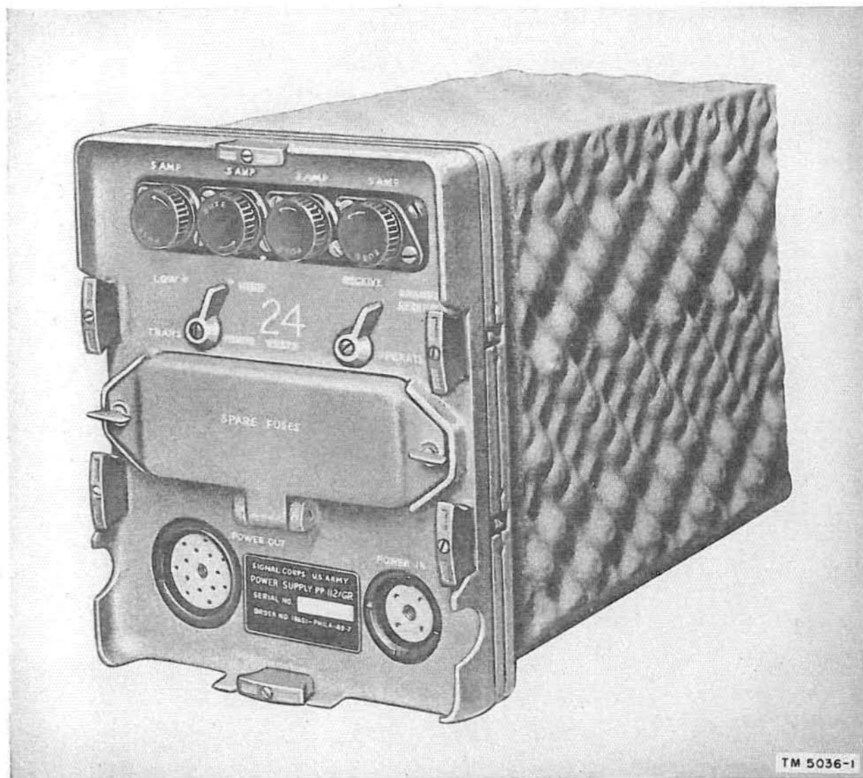
Figure 5. Power supply PP-112/GR, front view.
