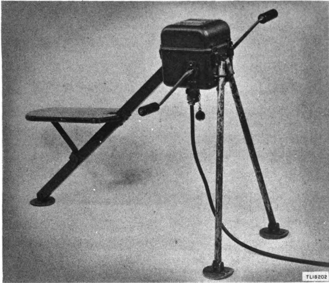
Figure 16. Generator G-3/TRC-7, set up for operation.
