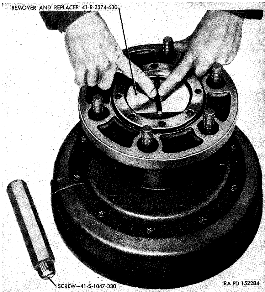
Figure 34. Fitting remover and replacer—41-R-2374-630 on bearing cup.
