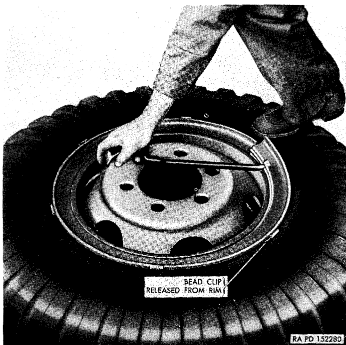
Figure 30. Prying lock ring from wheel.
