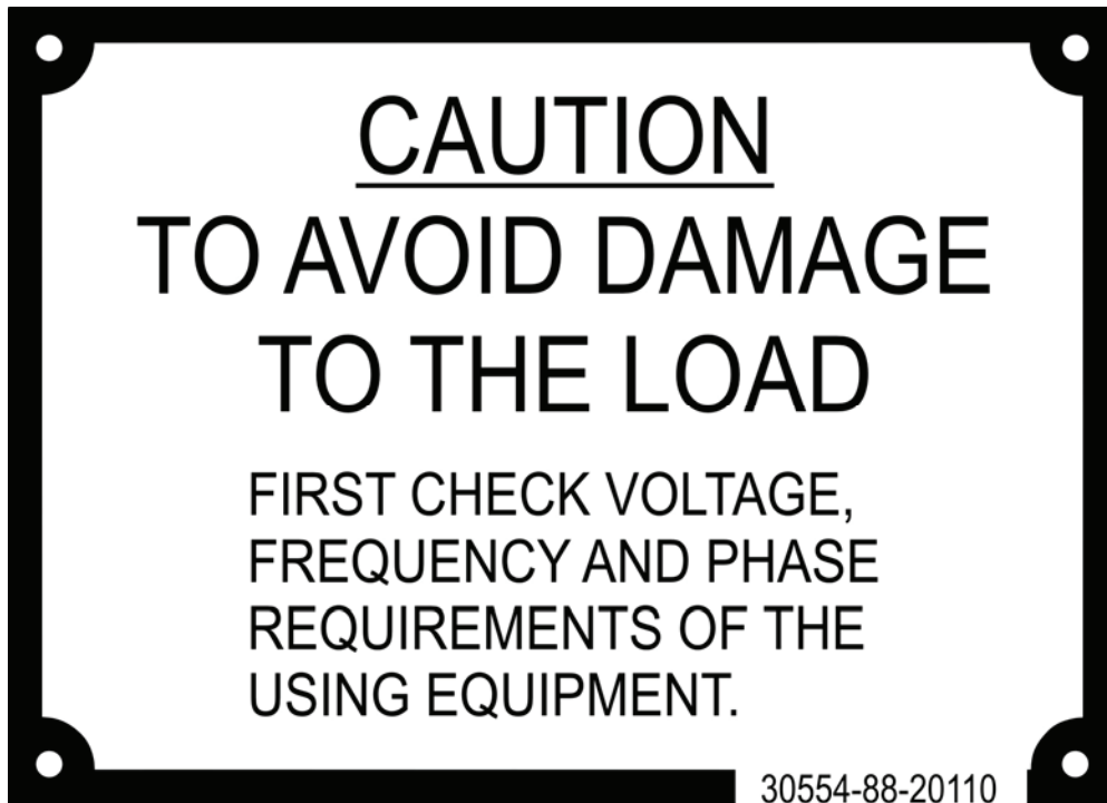
Figure 49. Label, Caution, Voltage Connection — Model 1050/1051.
