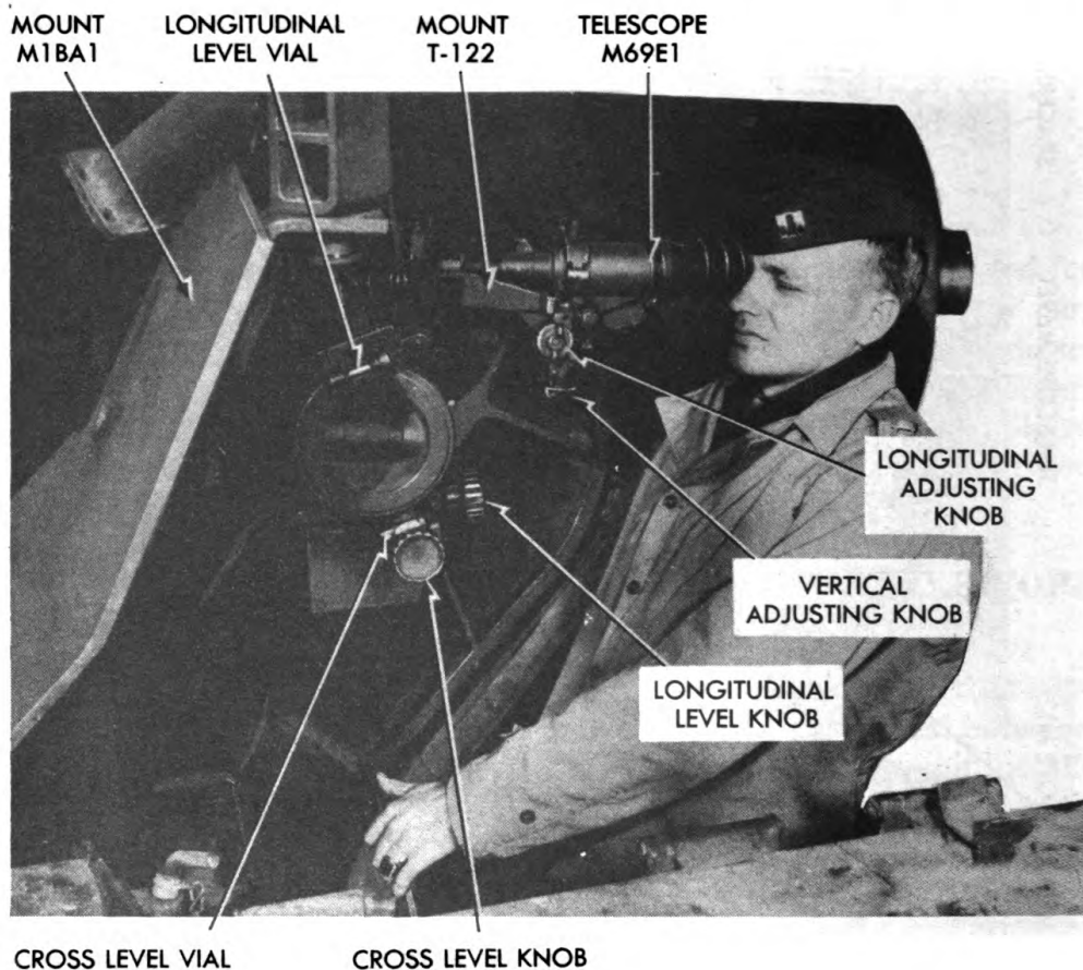
Figure 93—Sighting Equipment on Left Trunnion for 155-mm Gun Motor Carriage T83—Side View
