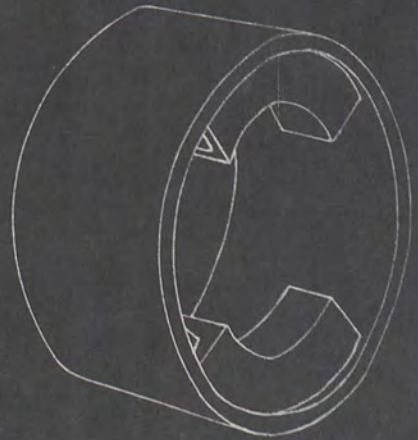
Dynamo's yoke and pole pieces.
