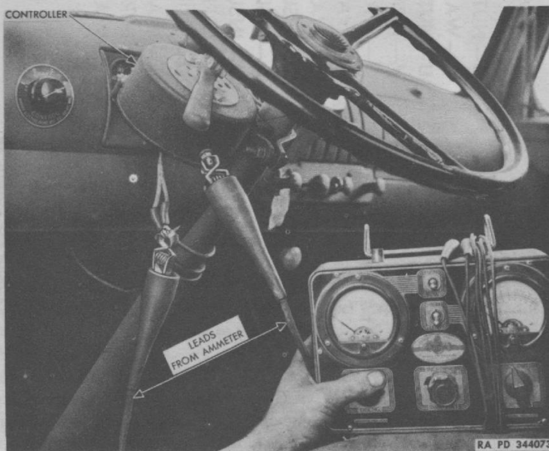
Figure 30—Checking Amperage at Controller
