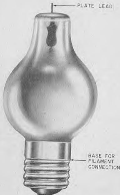
Figure 187. Tungar rectifier and bulb.
