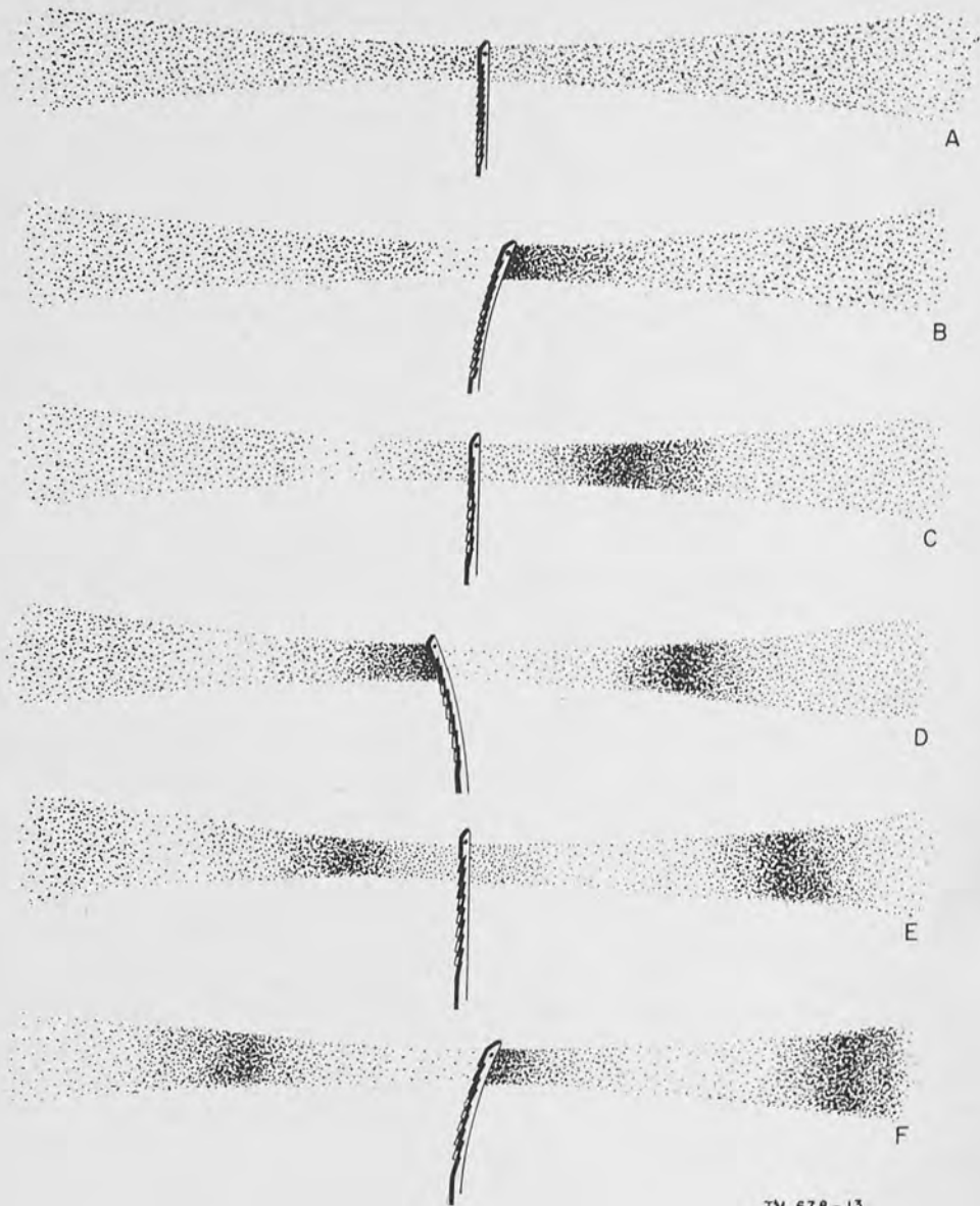
Figure 3. Sound wave produced by vibrating blade.
