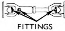
A — Short-Coupled Propeller Shaft Universal Joints. Lubricate, from under chassis, until oil shows through safety valve.
