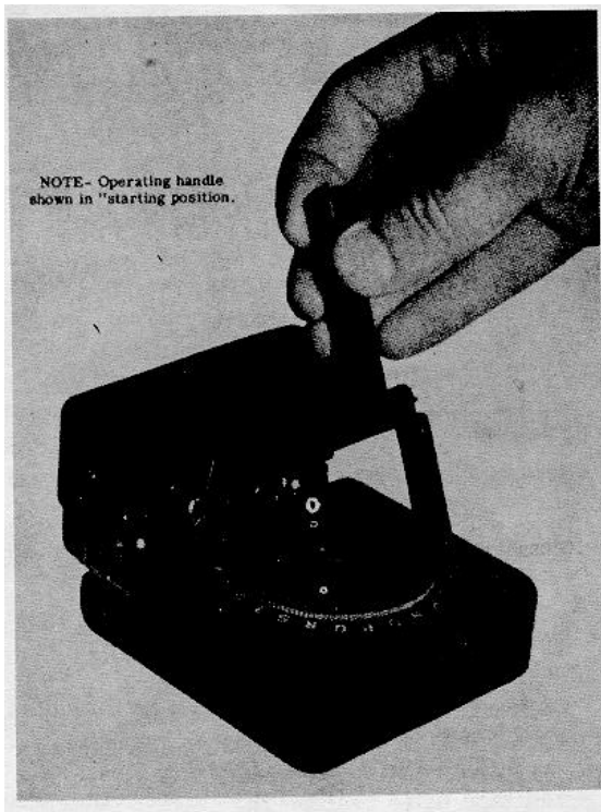
Figure 2-1. Using CO/B-8 Coder.
