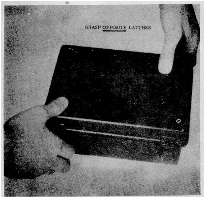
Figure 2-3. Removing KA-3 Keyer Adapter cover.
