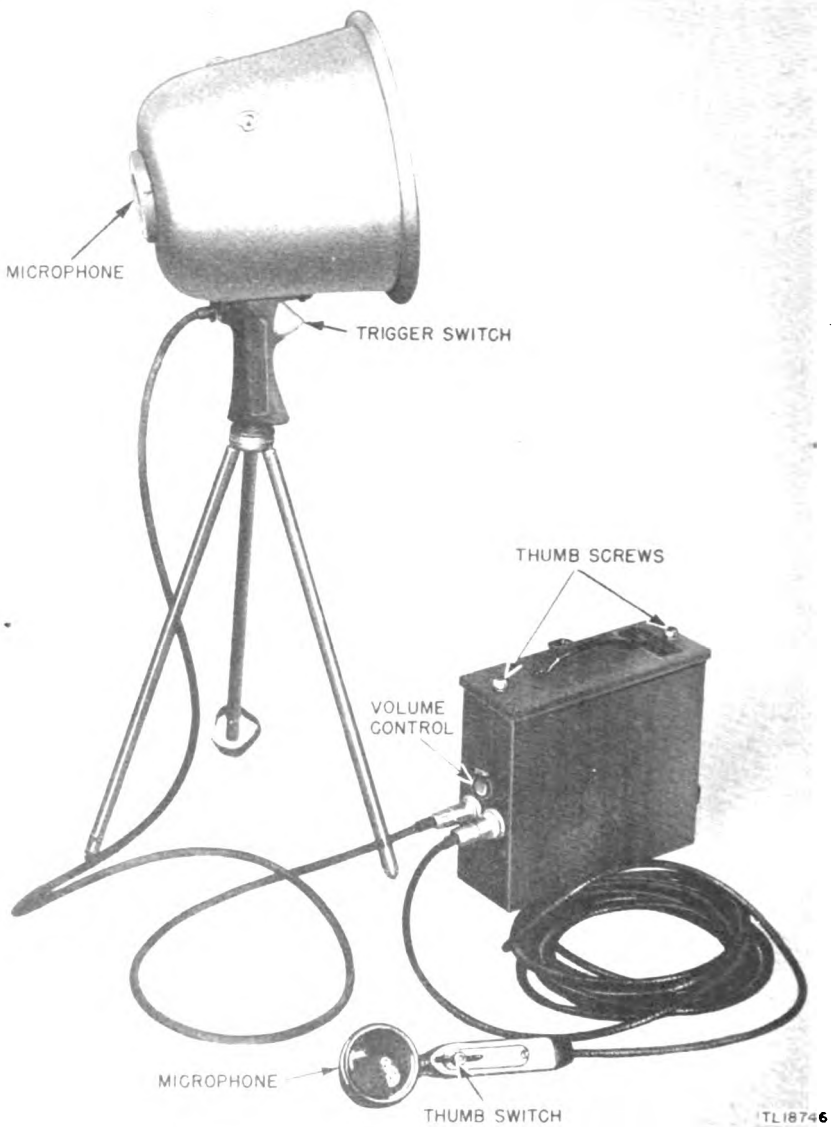
Figure 2. Public Address Equipment PA-4-C, assembled with Tripod M-230 and Microphone T-36-C
