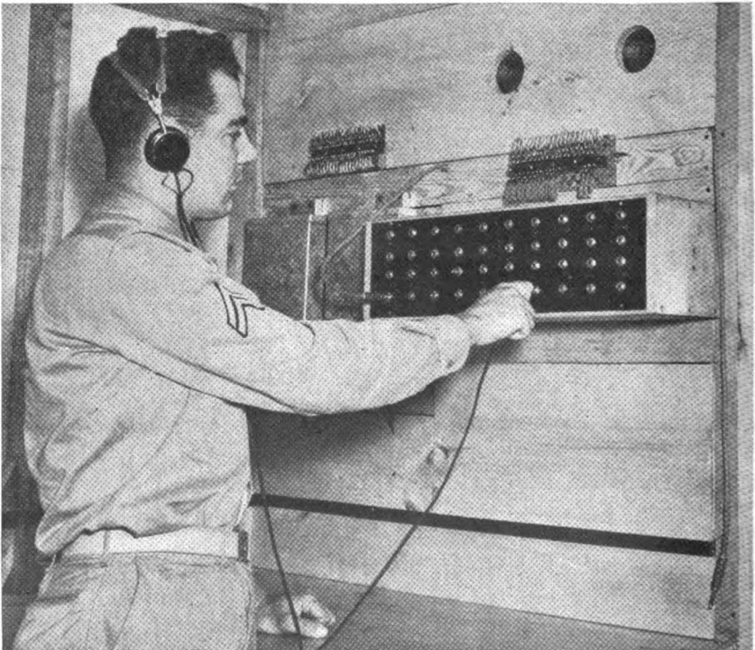
FIGURE 51.—Monitoring board used in connection with automatic keyers.
