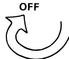
Turn the buzzer volume control clockwise until it stops to prevent any buzzer sound.
