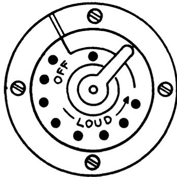
The buzzer volume control is located on the handset cord end of the telephone set.
