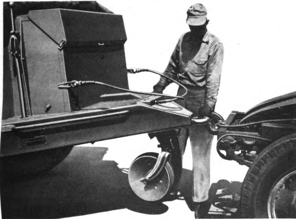
Figure 8—Coupling Trailer to Towing Vehicle
