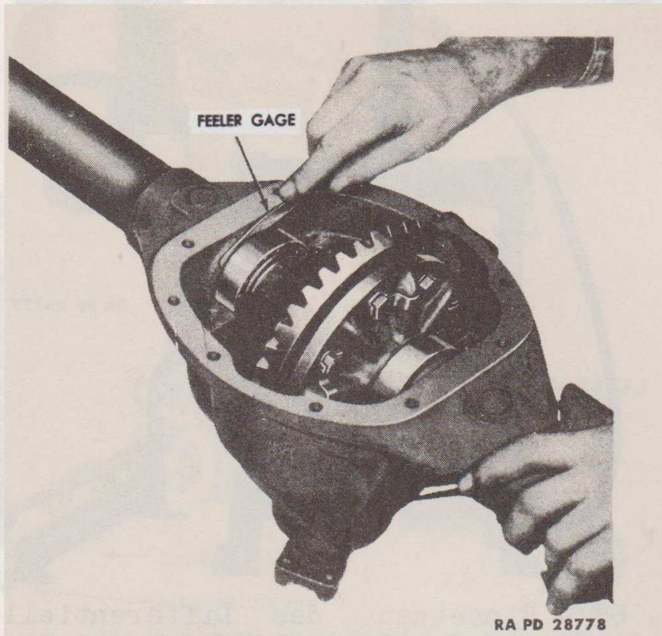
Figure 69—Checking Clearance Between Differential Case and Bearing
