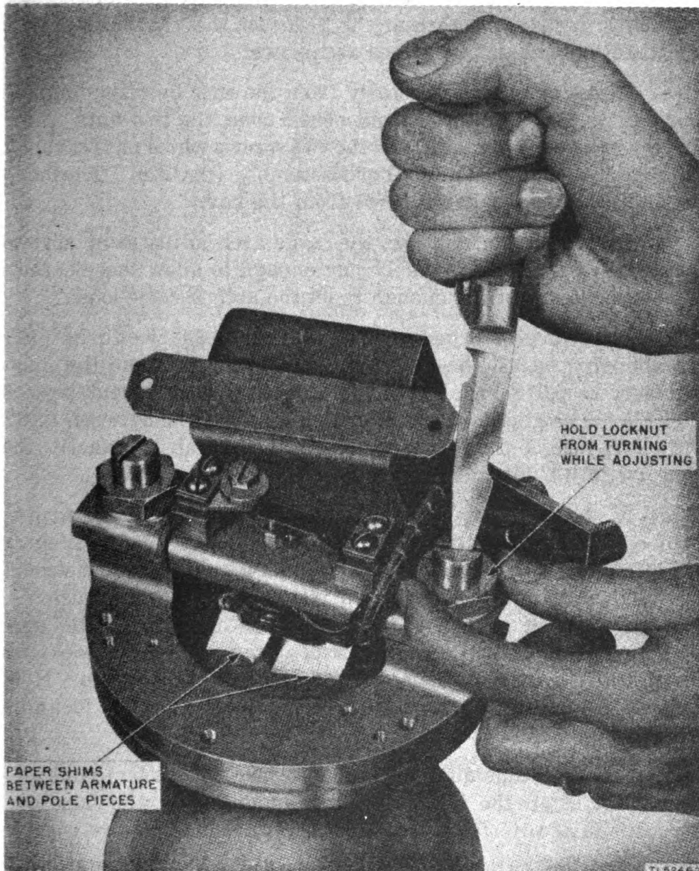
Figure 23. Adjusting armature gap on horn.
