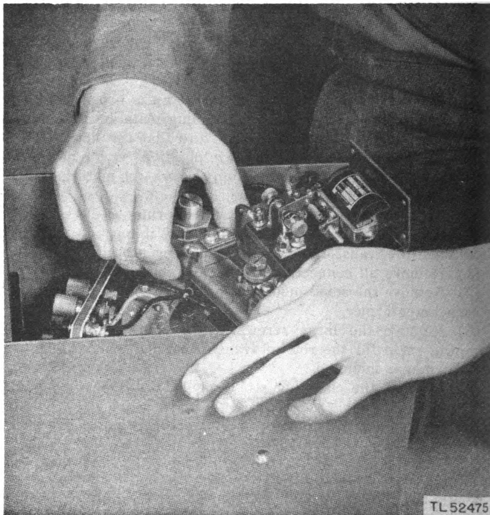
Figure 40. Replacing horn in case.
