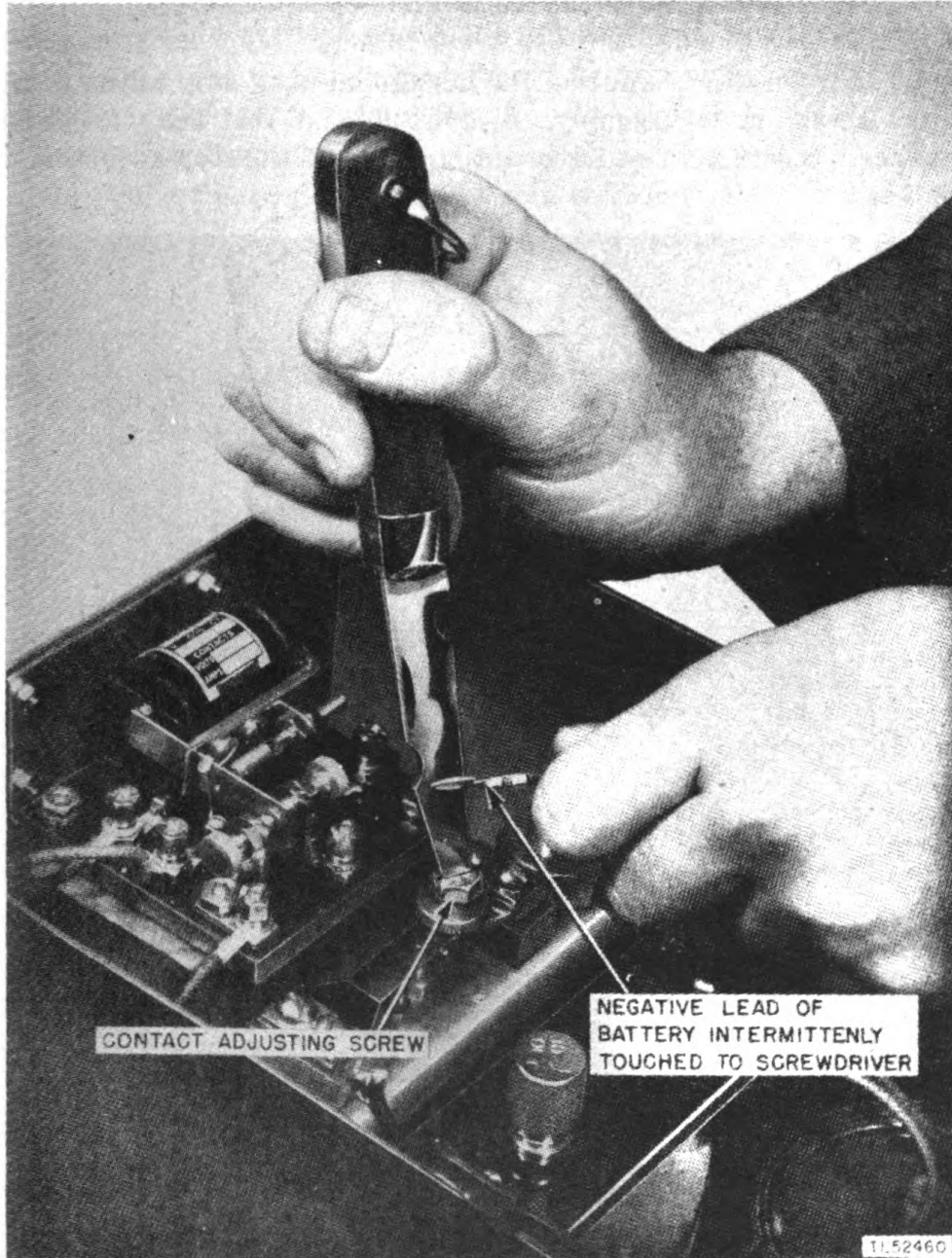
Figure 21. Adjusting horn contacts.
