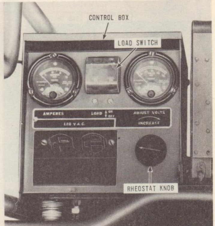
STEP 2. TURN RHEOSTAT KNOB FULLY COUNTERCLOCKWISE AND POSITION LOAD SWITCH TO OFF.
