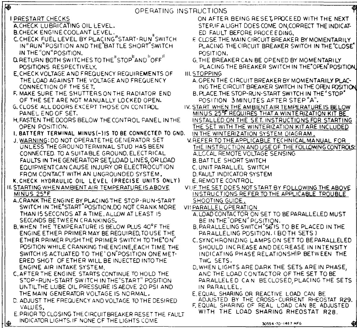
Figure 1-6. Operating Instructions Instruction Plate ME 6115-545-12/1-6 C3
