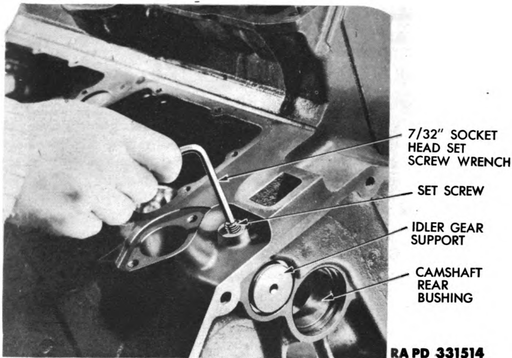
Figure 34 — Removing Set Screw For Idler Gear Support
