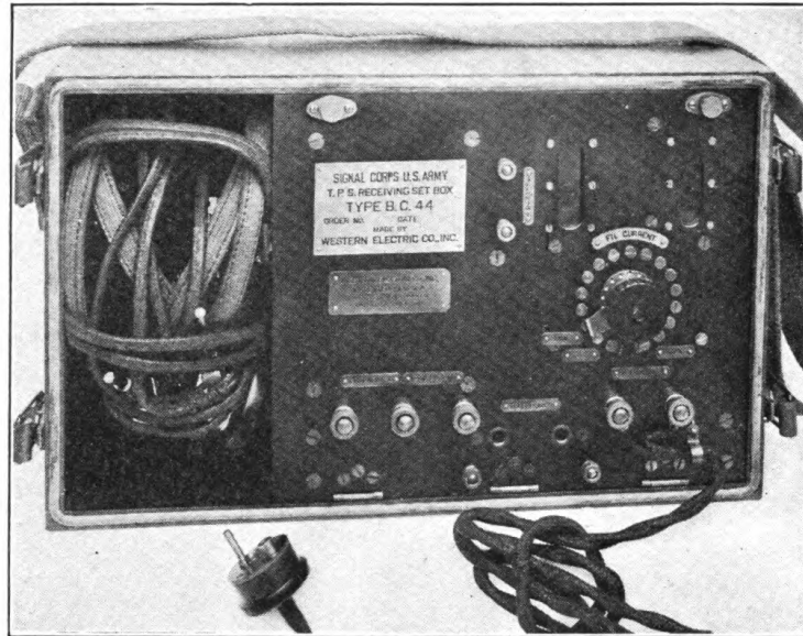
FIG. 2.—AMPLIFIER SET BOX, TYPE BC-44, FRONT VIEW.
