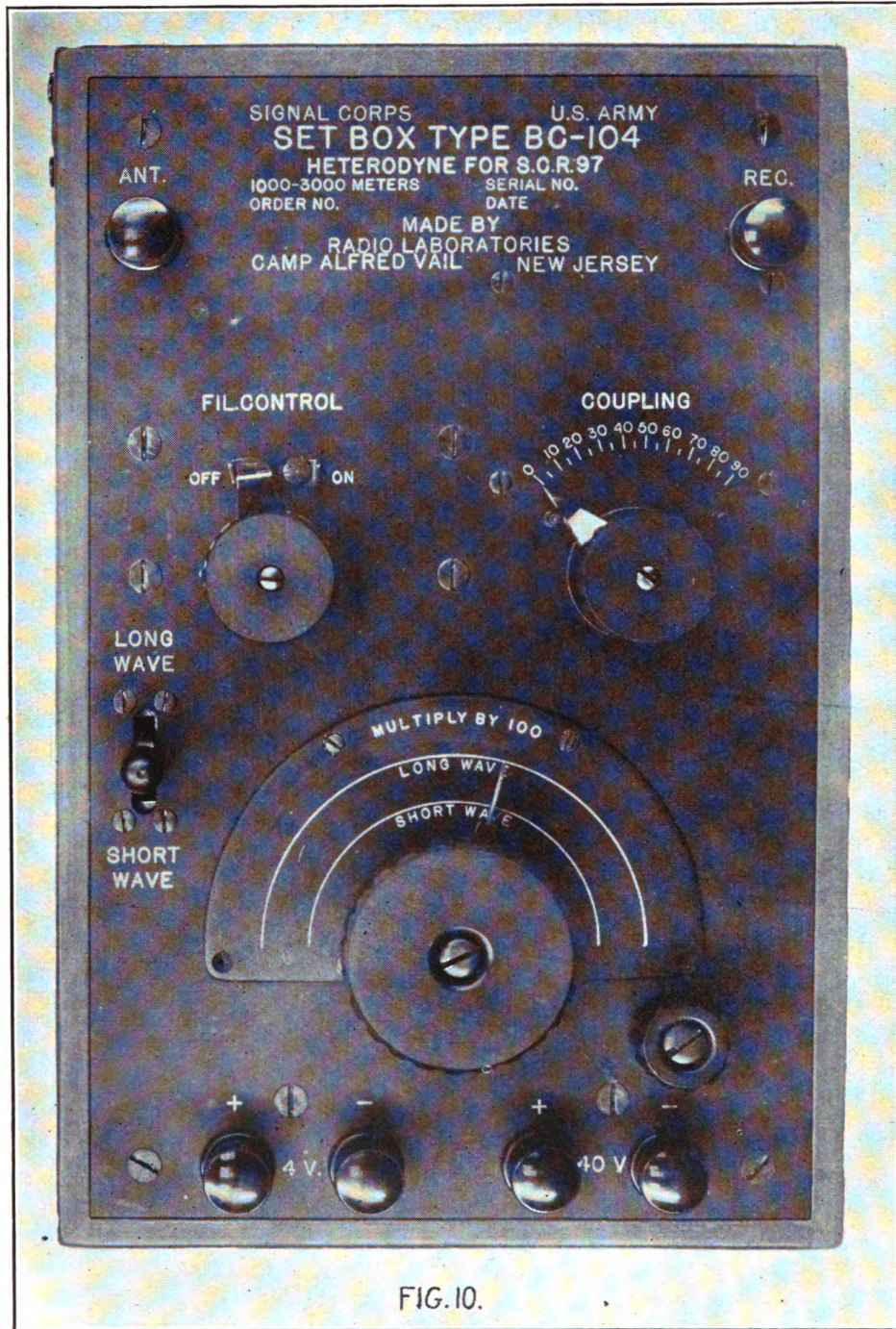
HETERODYNE SET BOX, TYPE BC-104, FRONT VIEW.
