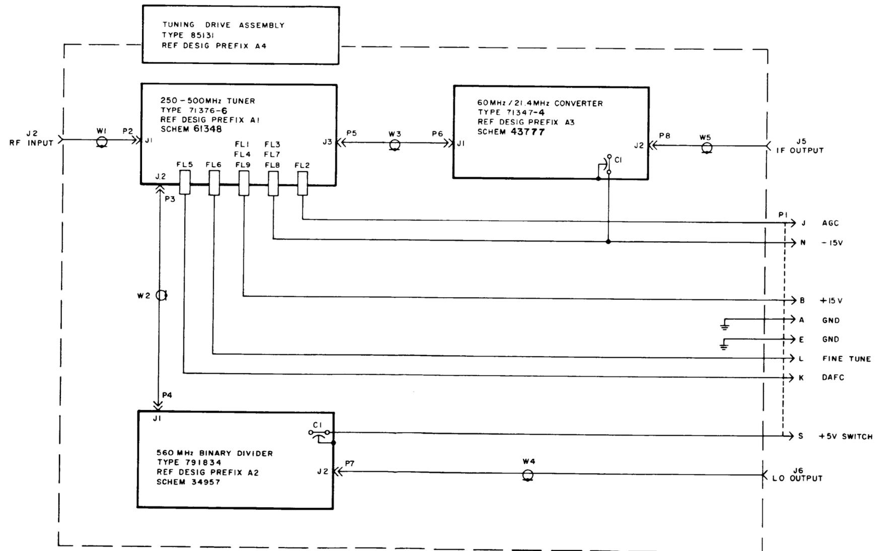
Figure 6-6. Type WJ-9124 250 - 500 MHz Tuner Assembly, Main Chassis, Schematic Diagram 43616
