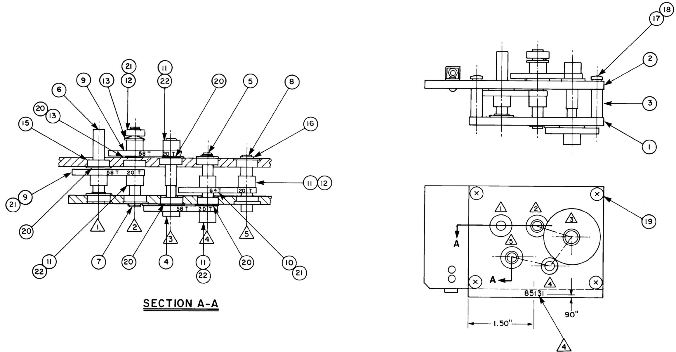
Figure 5-14. Type 85131 Tuning Drive (a4), Location of Components
