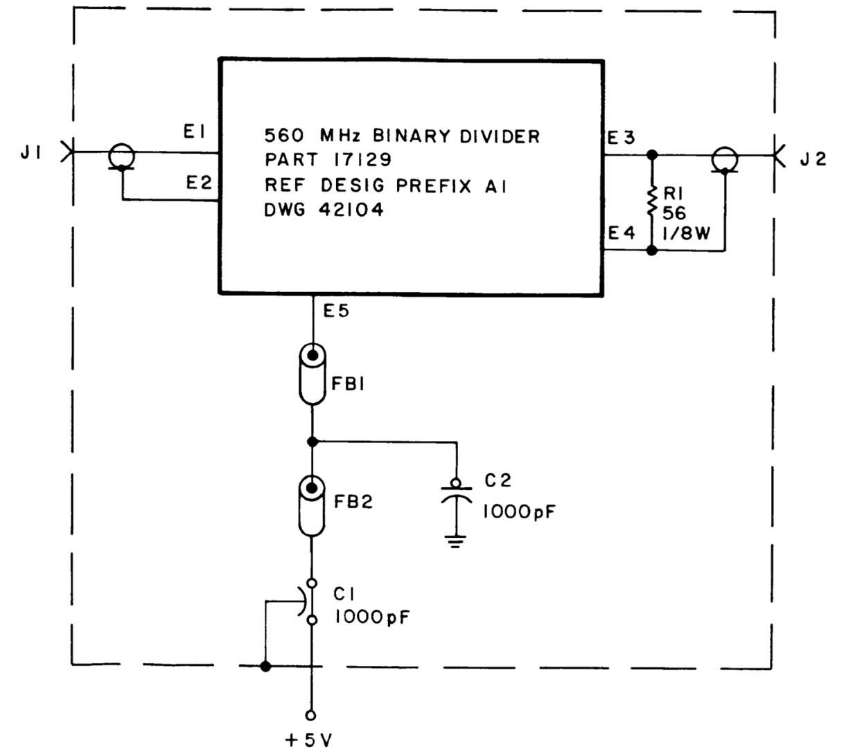
Figure 6-3. Type 791834 560 MHz Binary Divider (A2), Schematic Diagram 34957
