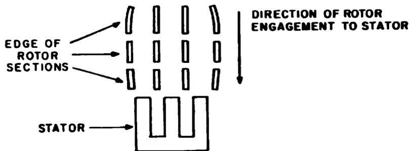
Figure 4-14. Rotor Plate Adjustment
