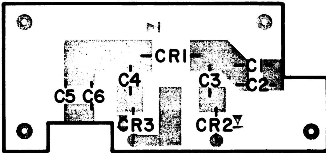
Figure 5-7. Part 17083 Pin Diode Attenuator (A1A1), Location of Components
