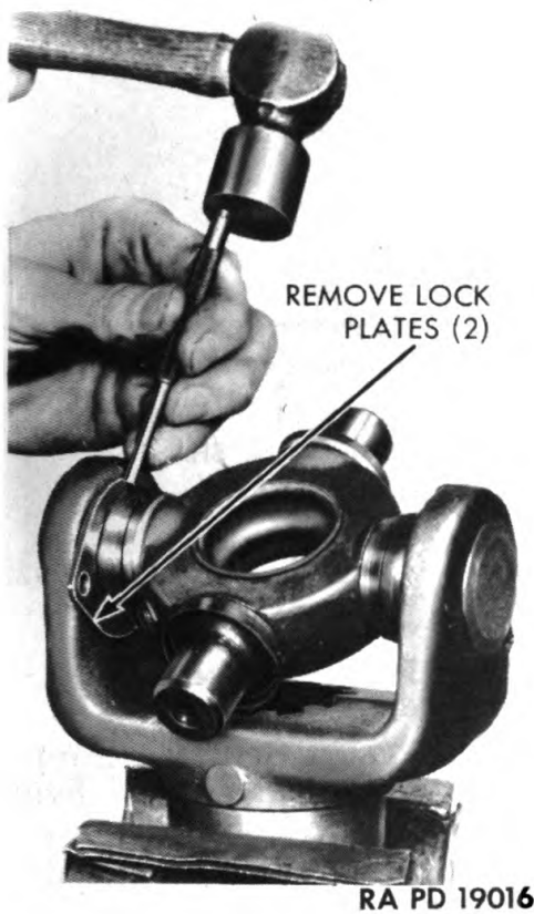
Figure 92 — Removing Trunnion Bearing Lock Plate
