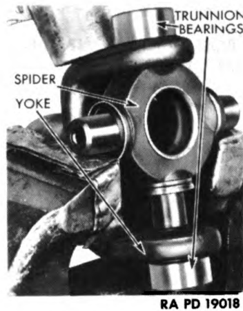
Figure 93 — Loosening Opposite Round Trunnion Bearing
