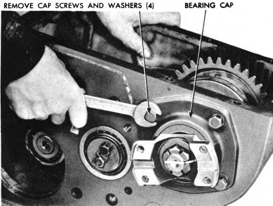
Figure 162 — Removing Transfer Case Front Axle Drive Shaft Front Bearing Cap Screws
