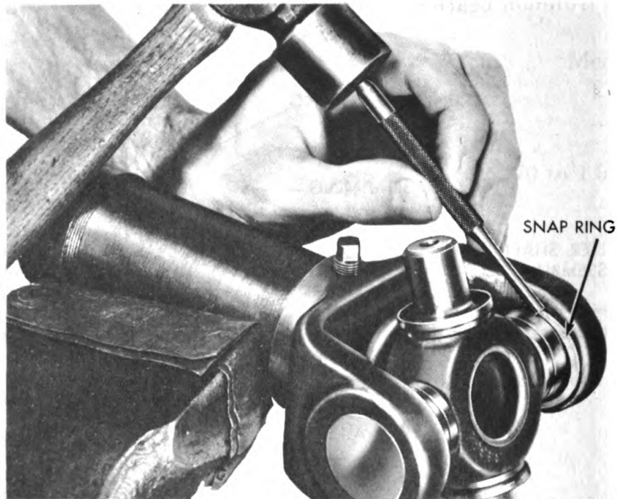
Figure 85 — Removing Round Trunnion Bearing Snap Ring
