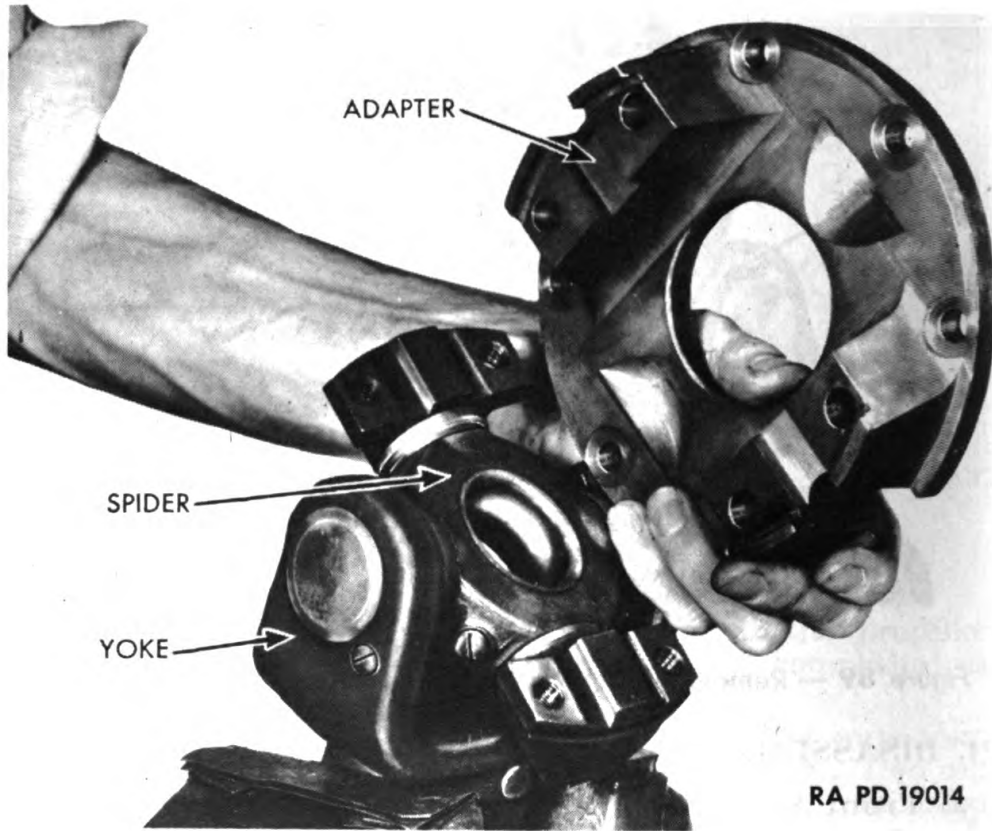
Figure 90 — Removing Rear Axle Propeller Shaft Adapter and Flanged Trunnion Bearings
