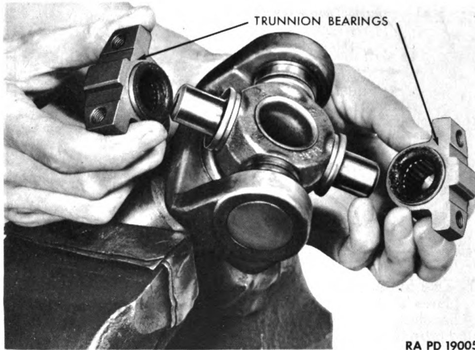
Figure 84 — Removing Flanged Trunnion Bearings
