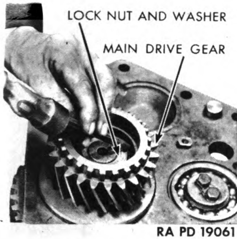
Figure 139 — Removing Transmission Main Drive Gear Lock Washer
