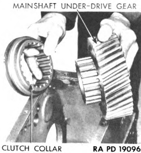
Figure 174 — Removing Drive Gear and Clutch Collar
