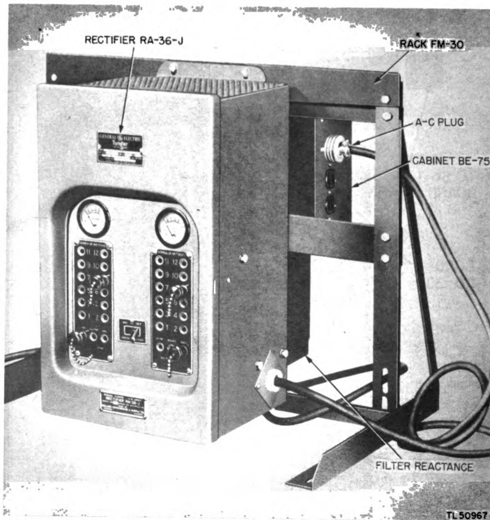
Figure 7. Rectifier RA-36-J mounted on Rack FM-30, front view.
